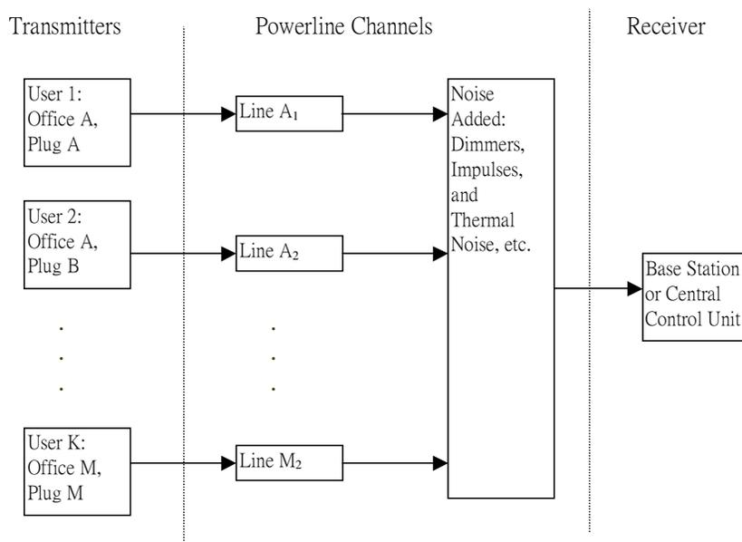
Fig. 1 Block diagram for MC-CDMA based power line communication systems.
