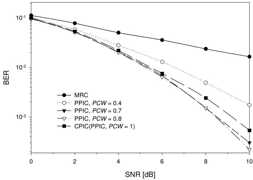
Fig. 7. The BER vs. SNR for two-stage PPIC detector with Gold codes,  $K = 12$ .
