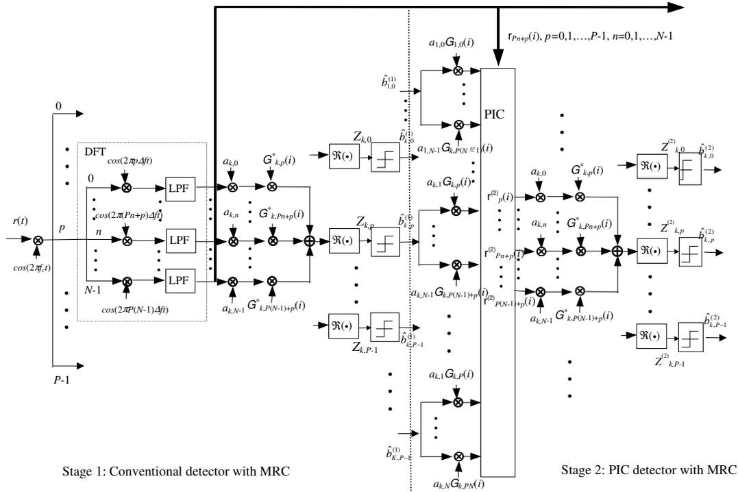
Fig. 4. Multistage parallel interference cancellation detection scheme with MRC for MC-CDMA PLC systems.
