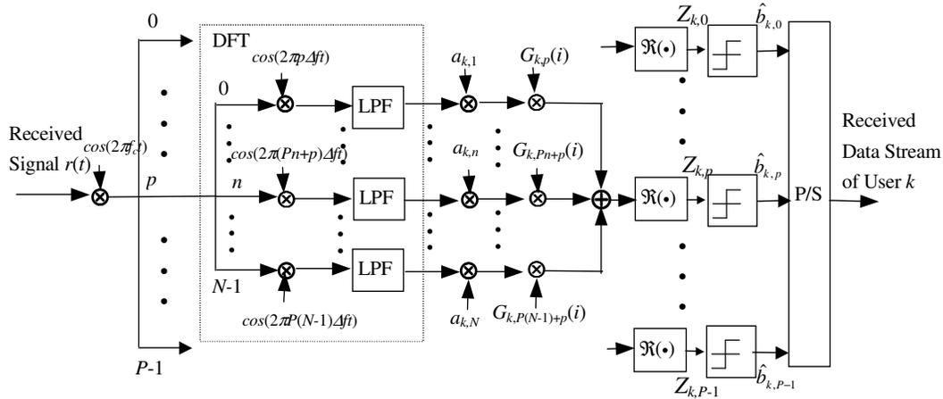
Fig. 3. Block diagram of MRC receiver for MC-CDMA communication systems.
