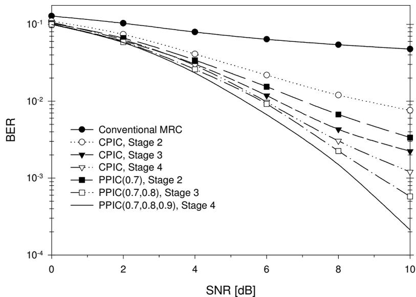
Fig. 9. Performance of BER vs. SNR for four-stage PPIC detectors,  $K = 20$ .
