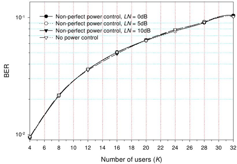
Fig. 5. Performance of MRC receivers with Gold codes for non-perfect power control over power line channels.
