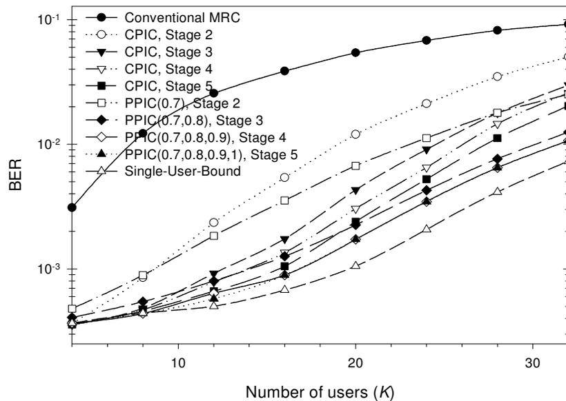
Fig. 10. Performance of BER vs. number of users for five-stage PPIC detectors,  $SNR = 8$  dB.
