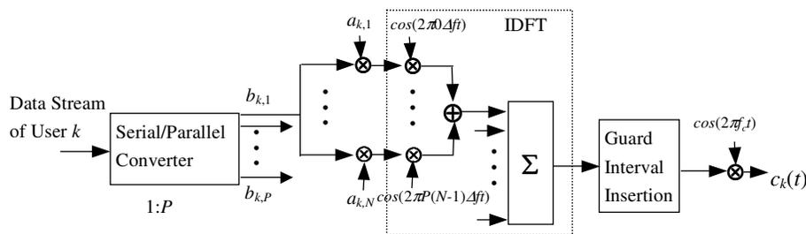
Fig. 2. Block diagram of transmitter for MC-CDMA PLC communication systems.
