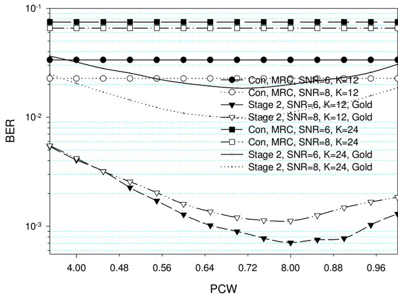
Fig. 6. Comparisons of BER vs. PCW for two-stage PPIC detector over power line channels without power control.
