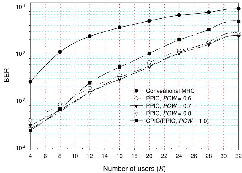
Fig. 8. The BER vs. number of users for two-stage PPIC detector with non-perfect power control power line channels,  $SNR = 6dB$ .
