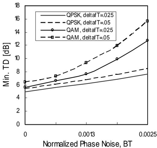
Fig. 4. Min. TD versus normalized linewidth for different values of normalized frequency offset for QPSK and 16QAM at BER=0.02.
