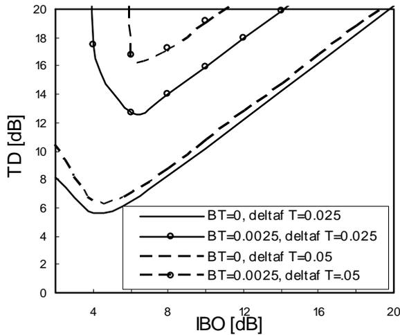
Fig. 3 .TD versus IBO for different values of normalized linewidth and normalized frequency offset for 16QAM at BER=0.02.
