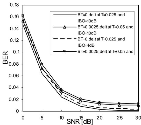
Fig. 1. BER versus SNR for QPSK under slowly Rayleigh fading channel for different values of normalized linewidth, frequency offset, and IBO.
