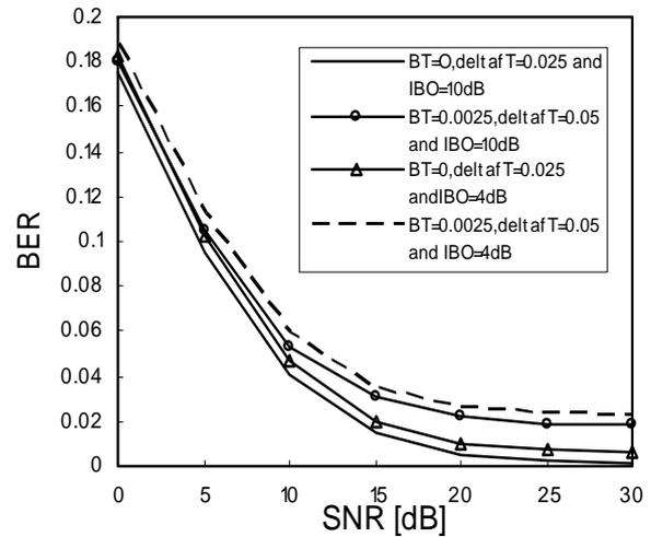
Fig. 2. BER versus SNR for QAM under slowly Rayleigh fading channel for different values of normalized linewidth, frequency offset, and IBO.
