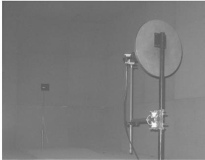
Fig. 13 Far-field pattern measurement of antenna in anechoic chamber.
