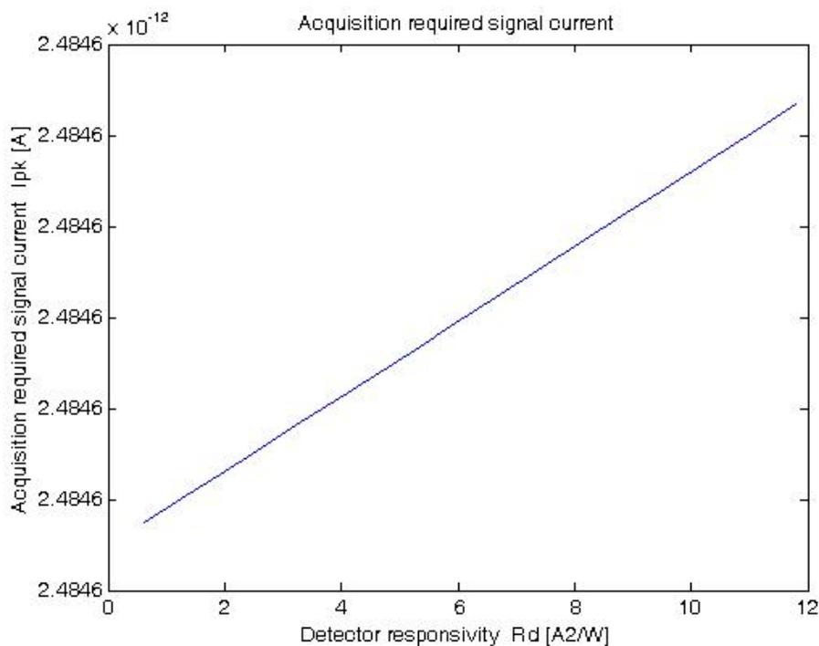
Fig. 4 Required signal current of acquisition link
