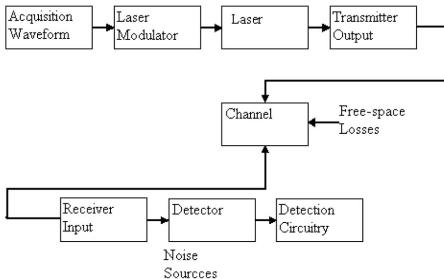
Fig. 3 Acquisition link model
