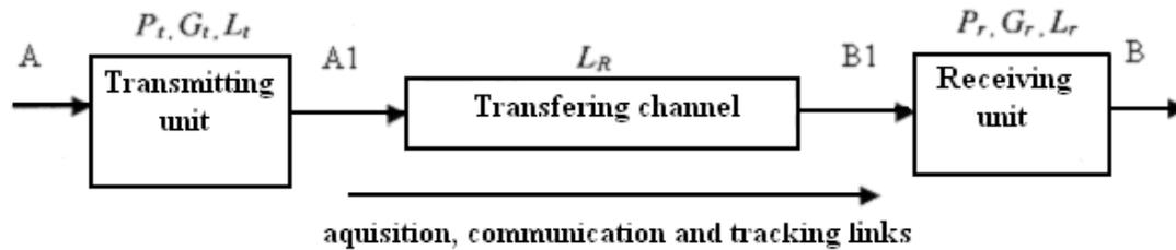
Fig.1 The model of signal transfer in LICS
