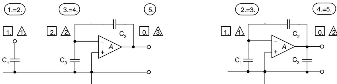
Fig.11. Diagrams of circuits for even and odd phases
