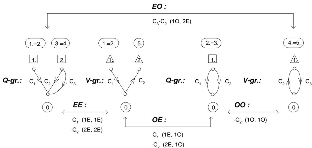
Fig.6. Two-graphs for even and odd phases
