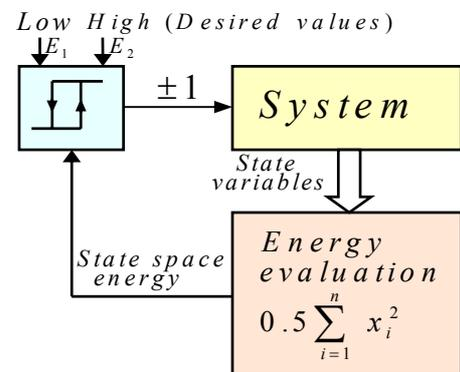
Fig. 9. Structure of state space energy controlled feedback system.
