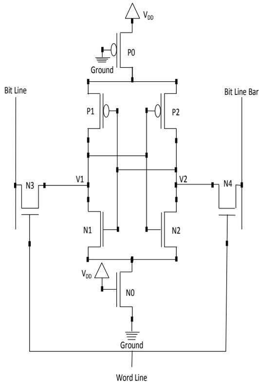
Fig. 3a: Modified 6T SRAM architecture
