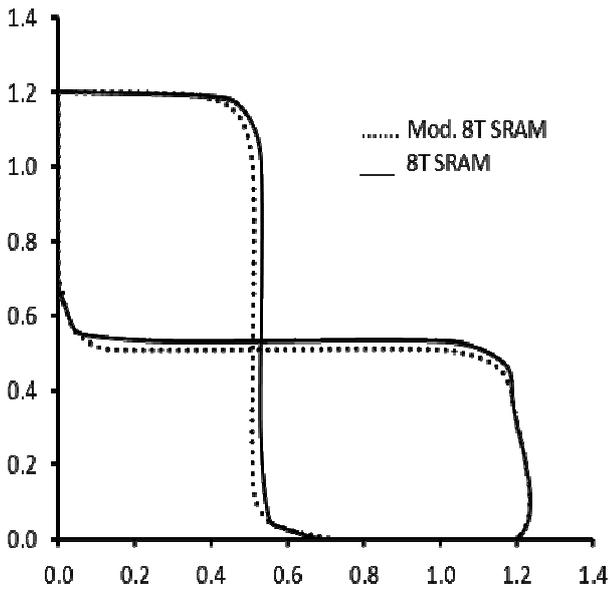
Fig. 5c: Butterfly curve for 8T-10T (modified 8T with transmission gate) SRAM architecture with transmission gate in place of access transistor
