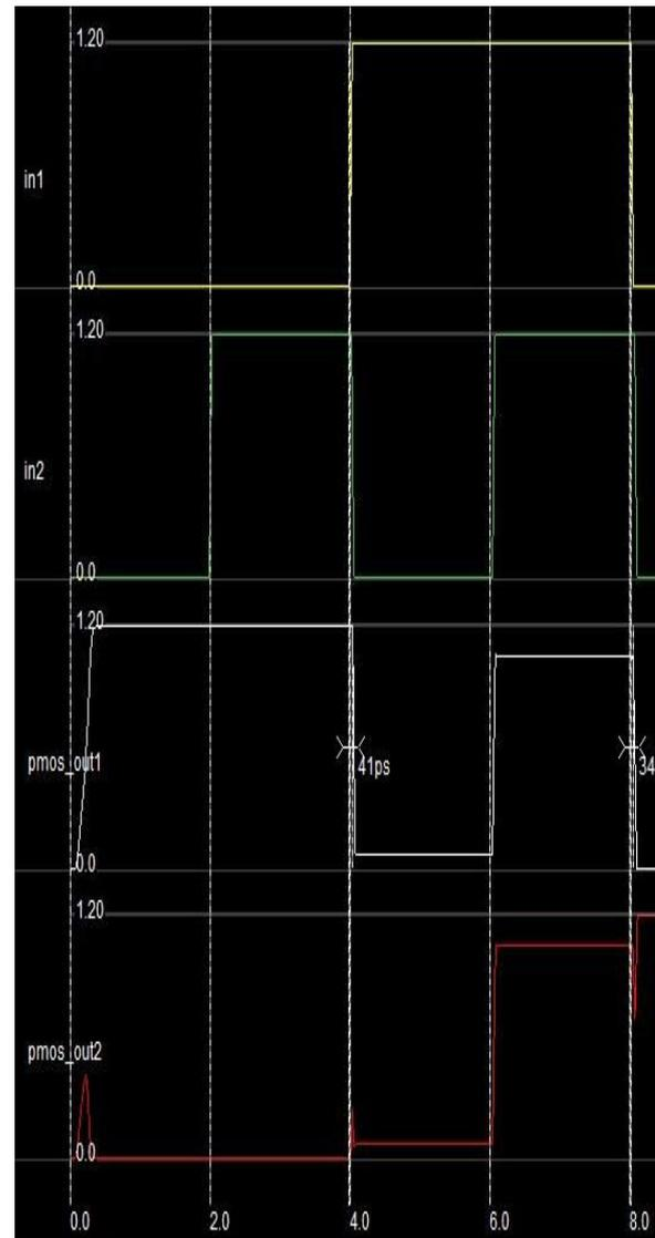
Fig. 5e: Simulation results for 10T-SRAM (modified 8T with transmission gate) architecture with transmission gate in place of access transistor
