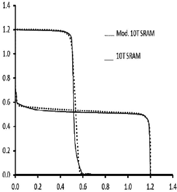
Figure 4c: Butterfly curve of 10T and modified 10T SRAM architecture
