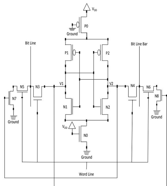
Fig. 4b: Modified 10T SRAM architecture
