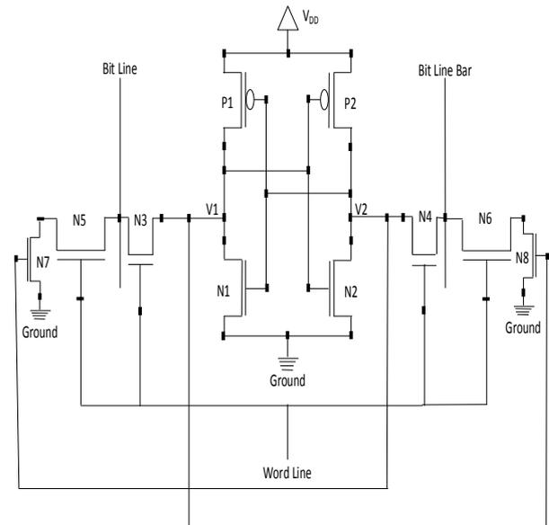
Fig. 4a: 10T SRAM architecture proposed by Sheshadri and Houston [2]
