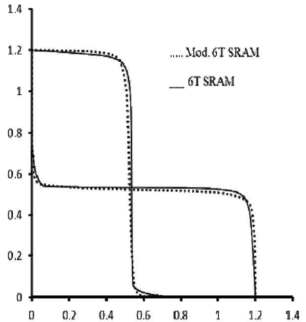
Fig.3b: Butterfly curves for 6T and 8T (modified 6T) SRAM architecture
