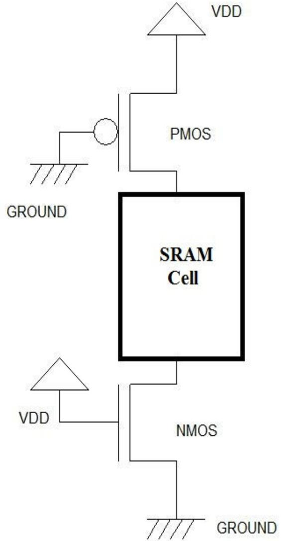
Fig. 2: Proposed technique for reducing write delay in SRAMs
