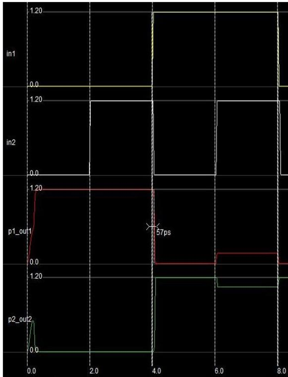
Fig. 4d: Simulation result for 10T-SRAM architecture with same  $V_T$  and W/L NMOSs
