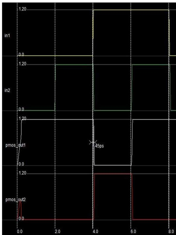
Fig. 5d: Simulation result for 8T-SRAM architecture with transmission gate in place of access transistor
