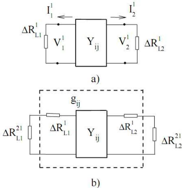
Fig.7. A traditional approach to recalculation of currents: a)- load resistors  $\Delta R_{L1}^1, \Delta R_{L2}^1$  are as increments concerning initial zero values; b)- the changes  $\Delta R_{L1}^{21}, \Delta R_{L2}^{21}$  are concerning values  $\Delta R_{L1}^1, \Delta R_{L2}^1$
