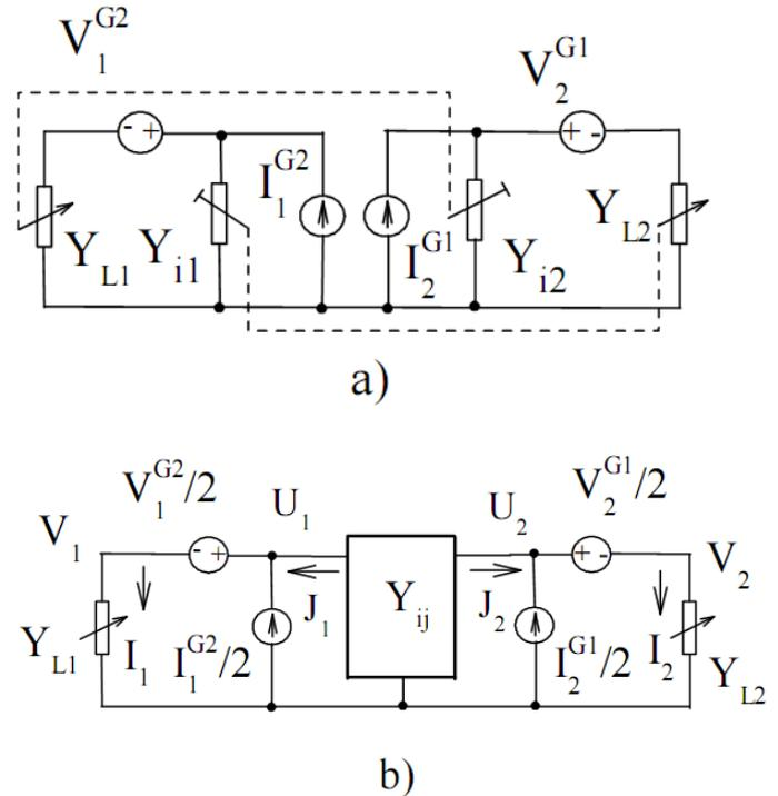
Fig.10. The proposed equivalent generator of the active two-port network: a)- is as an association of two active two-poles: b)-is as generalization of the equivalent generator of active two-port network
