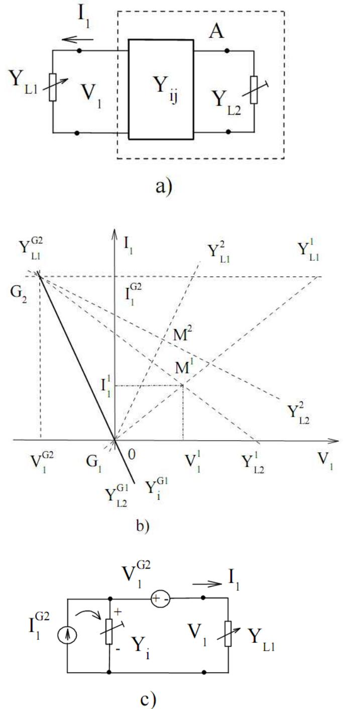
Fig.9. An active two-pole with a changeable element  $Y_{L2}$ : a)- scheme of this active two-pole; b)- family of load characteristics; c)- generalized equivalent generator
