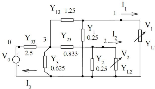
Fig.1. An active two-port network with changed conductivities of loads
