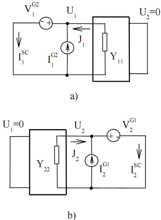
Fig.11. The definition of input conductivity of the passive two-port network: a)- at short circuit of the first load and short circuit of the second pair terminals; b)- at short circuit of the second load and short circuit of the first pair terminals
