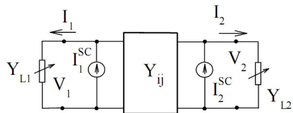
Fig.8. A traditional equivalent generator of an active two-port network
