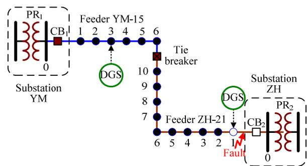
Fig.9 The connecting locations of the two DGS for the simulation scenario in subsection 4.3
