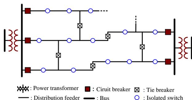
Fig. 1 A schematic configuration of a power distribution system
