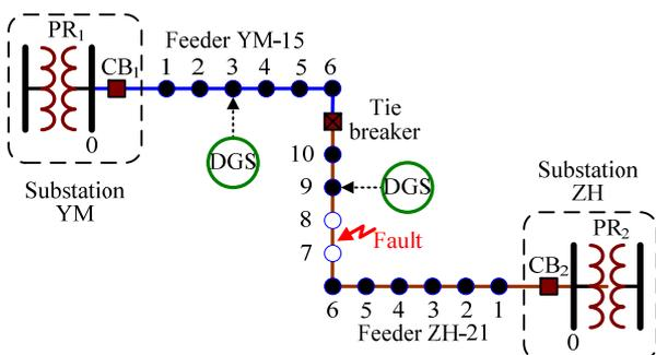
Fig.13 The connecting locations of the two DGS for the simulation scenario in subsection 4.5
