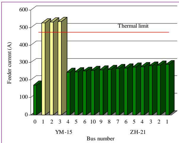
Fig.10 Current profiles of example feeder YM-15 and ZH-21 after load transfer
