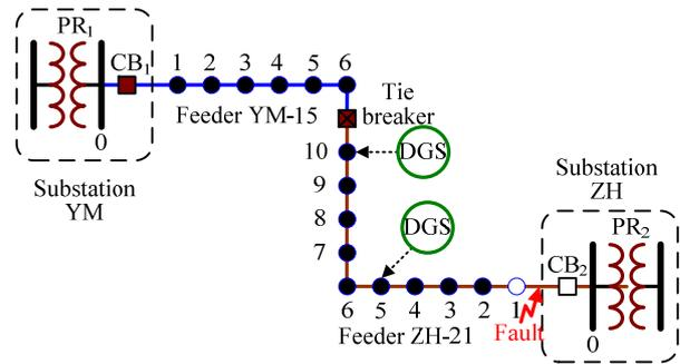
Fig.11 The connecting locations of the two DGS for the third simulation scenario in subsection 4.4
