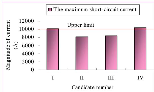
Fig.18 The maximum short-circuit currents of each load transfer candidate
