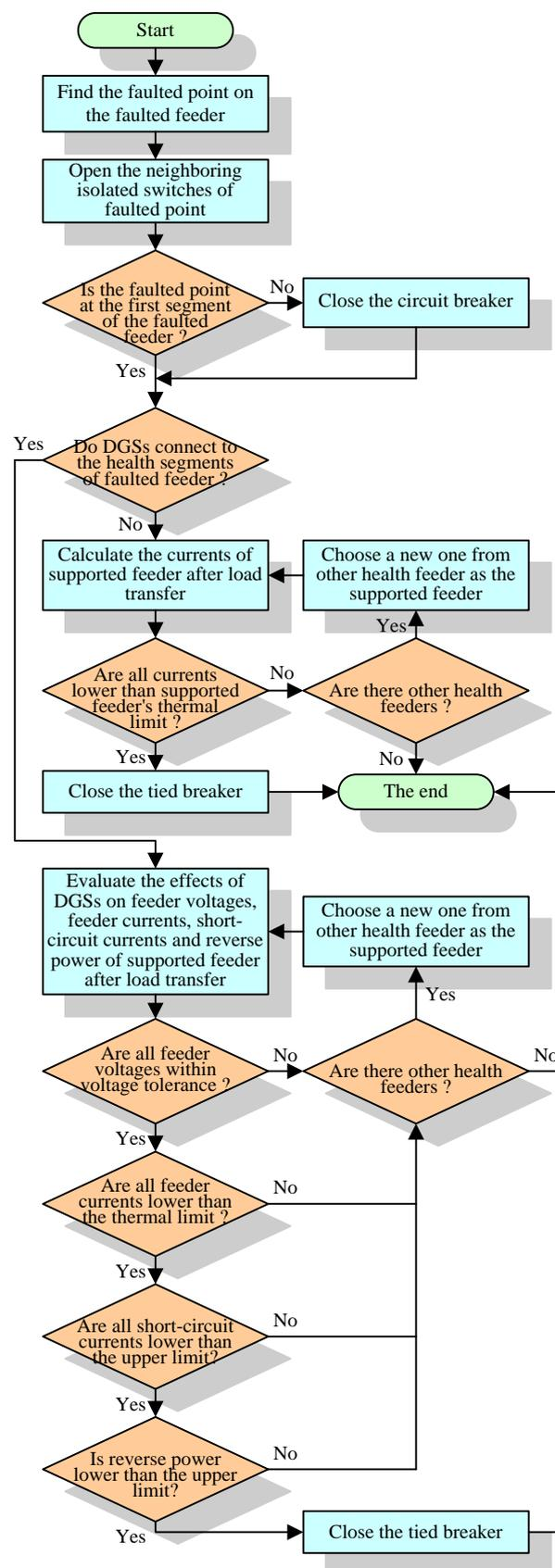
Fig. 3 Flowchart of proposed load transfer scheme
