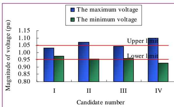
Fig.16 The maximum and minimum feeder voltages of each load transfer candidate
