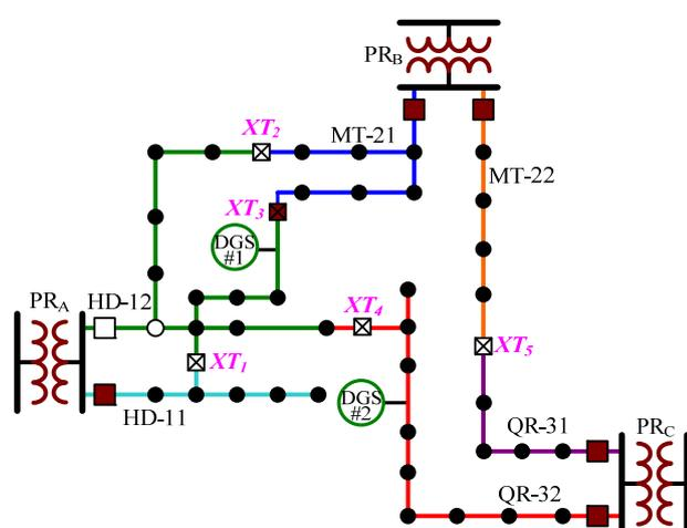
Fig.20 The new configuration of the example system II after load transfer
