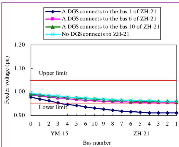
Fig.6 Voltage profiles of example feeders YM-15 and ZH-21 (DGS's power factor is 0.95 leading)
