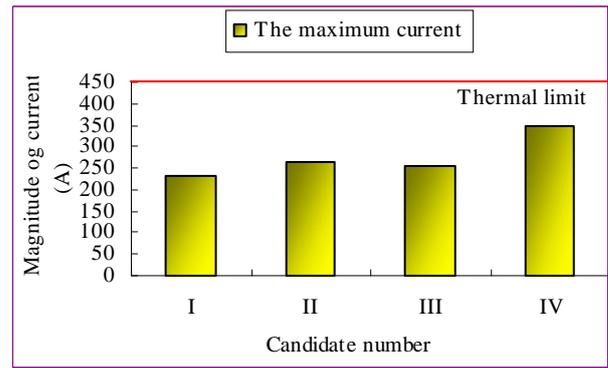
Fig.17 The maximum feeder currents of each load transfer candidate
