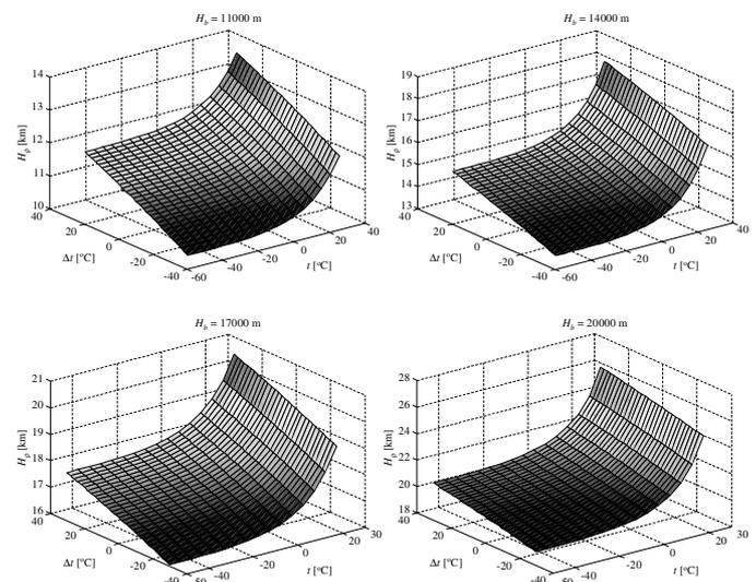
Fig. 10 Density altitude for layer 1 at the temperature and humidity variations
