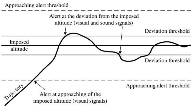
Fig. 1 Basic operation of the altitude alerting systems
