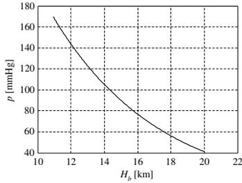
Fig. 4 Pressure variation with the altitude in the layer 1
