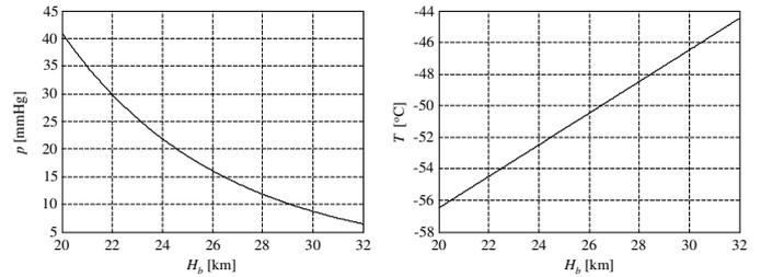
Fig. 5 Pressure and temperature variations with the altitude in the layer 2
