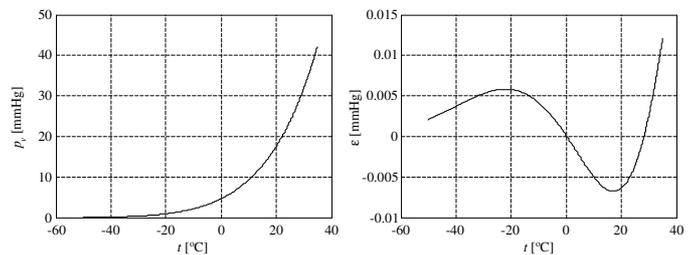
Fig. 7 Evaluation of formulas for calculating the vapor pressure
