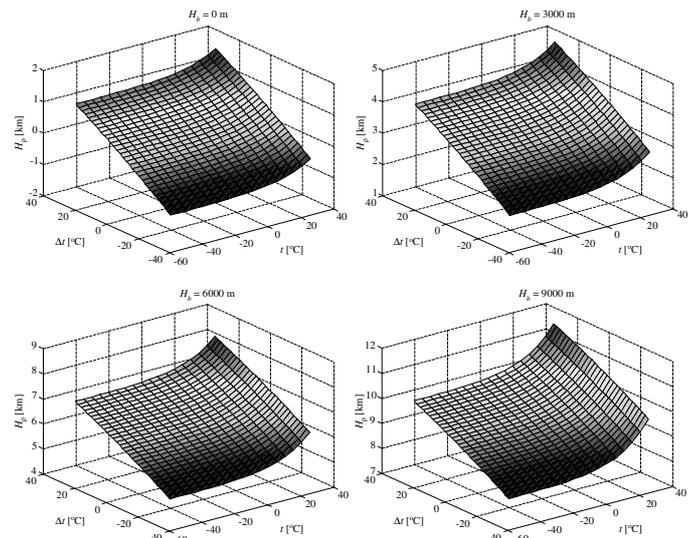
Fig. 8 Density altitude for layer 0 at the temperature and humidity variations
