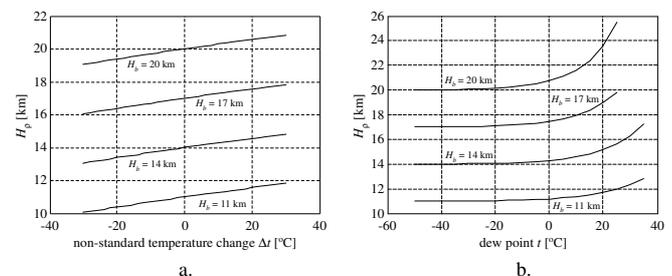
Fig. 11 The evaluation of the influences of the non-standard temperature variations and humidity on the density altitude in the layer 1
