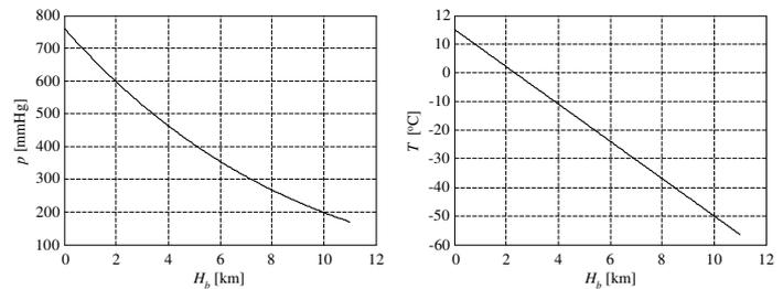
Fig. 3 Pressure and temperature variations with the altitude in the layer 0
