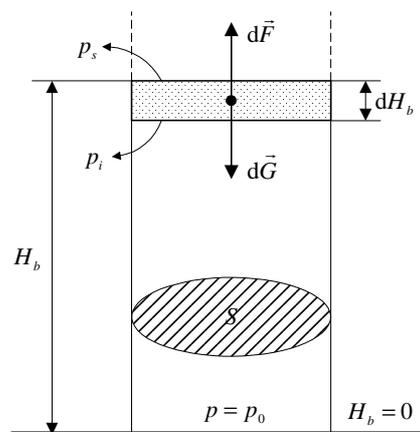
Fig. 2 Hydrostatic equilibrium of an air layer with infinitesimal thickness
