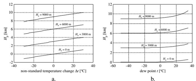
Fig. 9 The evaluation of the influences of the non-standard temperature variations and humidity on the density altitude in the layer 0
