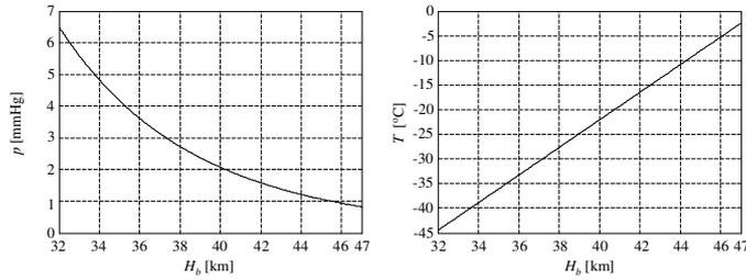
Fig. 6 Pressure and temperature variations with the altitude in the layer 3
