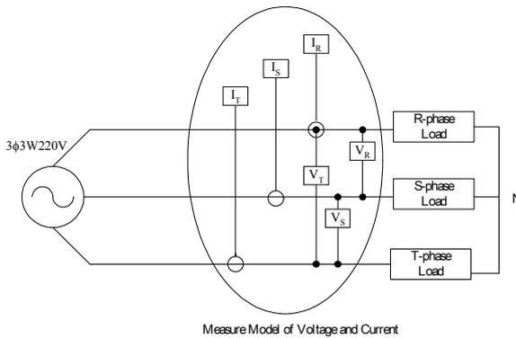
Figure 2. Three-Phase Three-Wire System
