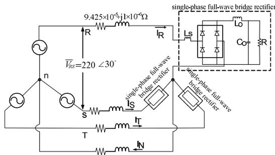
Figure 3. Three-Phase Four-Wire Simulation Model
