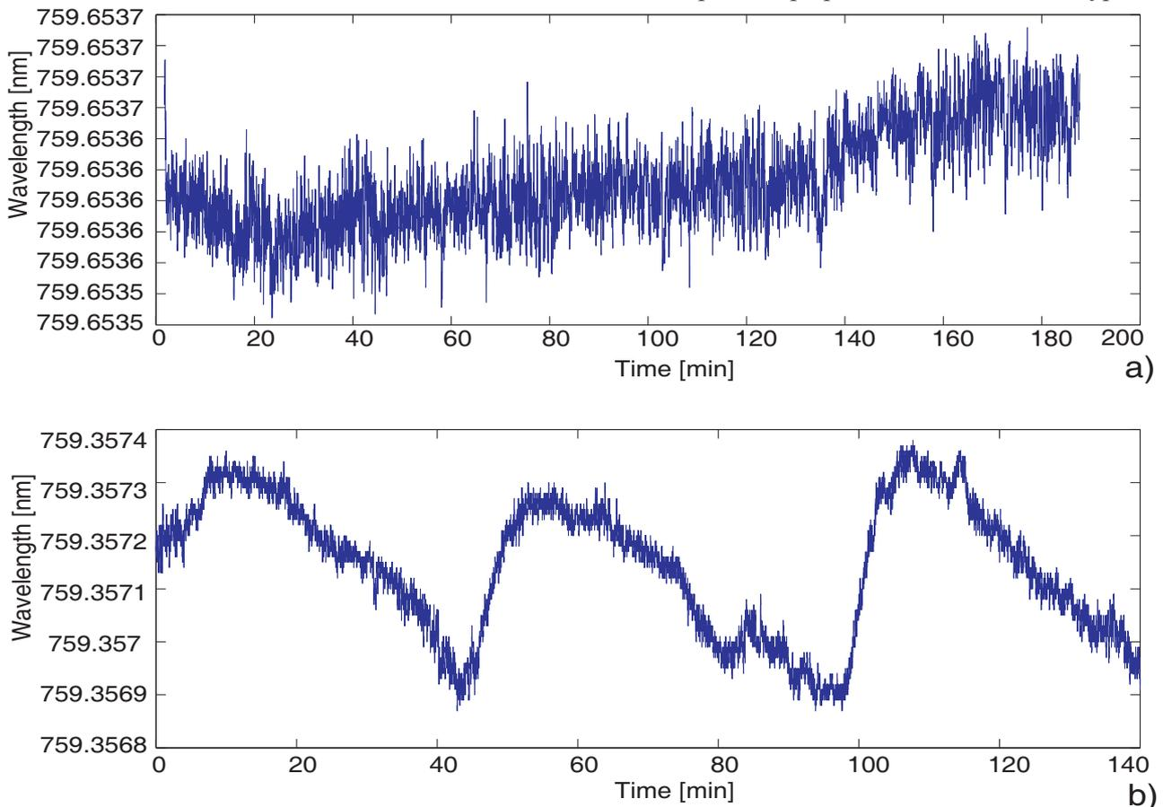
Fig. 3: Long time stability of the lasing wavelength of the a) DFB laser source, b) VCSEL laser source.
