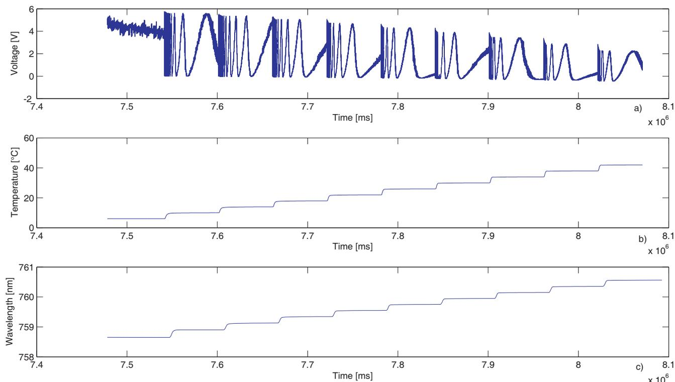
Fig. 4: The tunable range of the wavelength of the DFB laser diode by change of the temperature of the chip; a) The record from the F-P resonator - The number of passed resonance periods of a stable F-P resonator is 40 for each temperature step. b) The temperature of the chip. c) The wavelength of the DFB laser diode measured by lambdameter.
