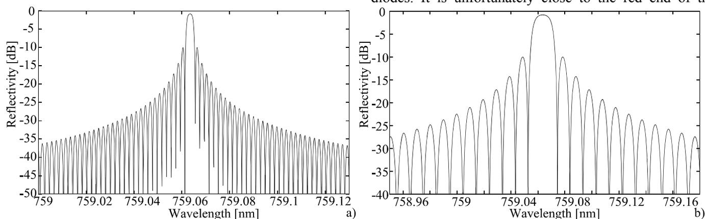
Fig. 6. Simulation of reflectivity spectral characteristics of uniform fiber Bragg gratings, a) 100 mm length fiber grating with refractive index change  $8 \times 10^{-6}$ , b) 20 mm length fiber grating with refractive index change  $4 \times 10^{-5}$ .
