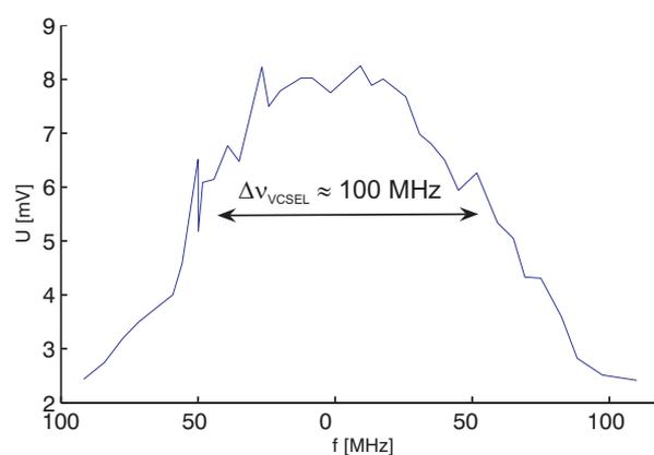
Fig. 1. Frequency beat between Ti-Sa laser and VCSEL diode.
