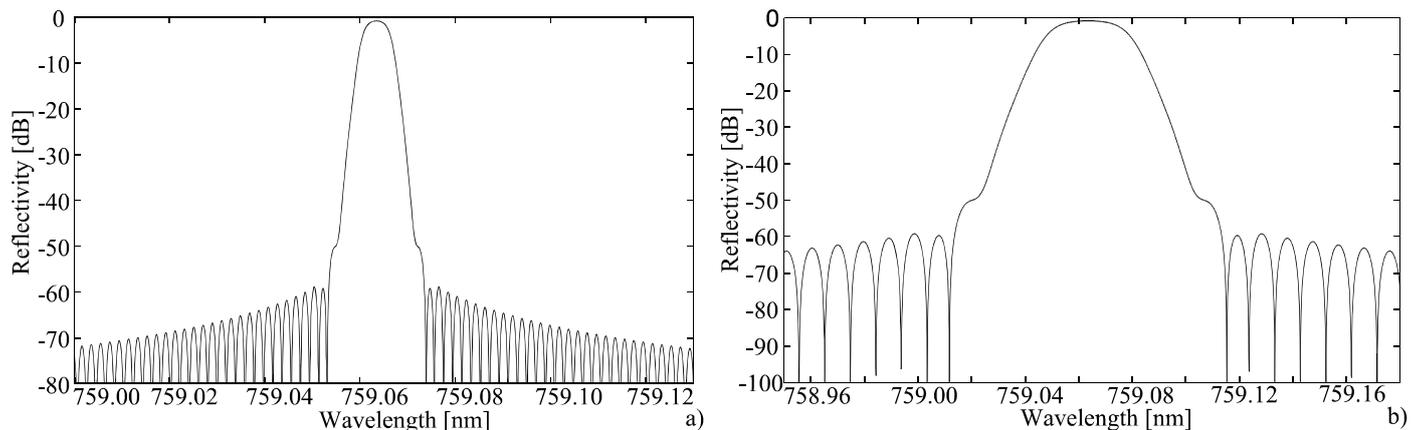
Fig. 7. Simulation of reflectivity spectral characteristics of Gaussian apodized fiber Bragg gratings, a) 100 mm length fiber grating with refractive index change  $2 \times 10^{-5}$ , b) 20 mm length fiber grating with refractive index change  $1 \times 10^{-4}$ .
