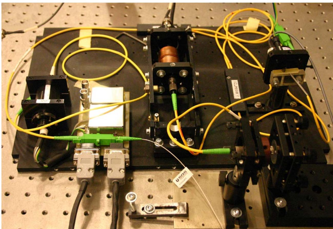
Fig. 11: Practical realization of the DFB laser source and the fiber laser interferometer.
