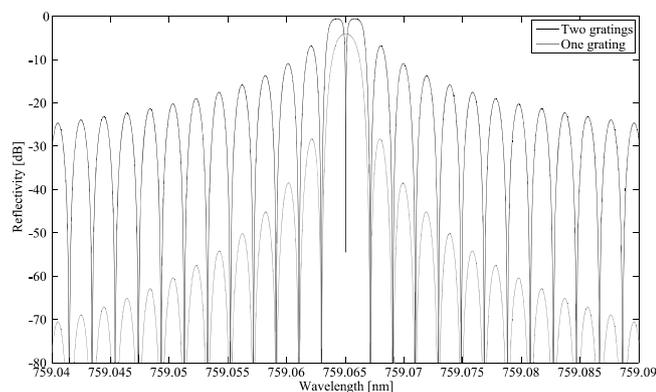
Fig. 8. Simulation of reflectivity spectral characteristics of Gaussian apodized multiple fiber Bragg grating.
