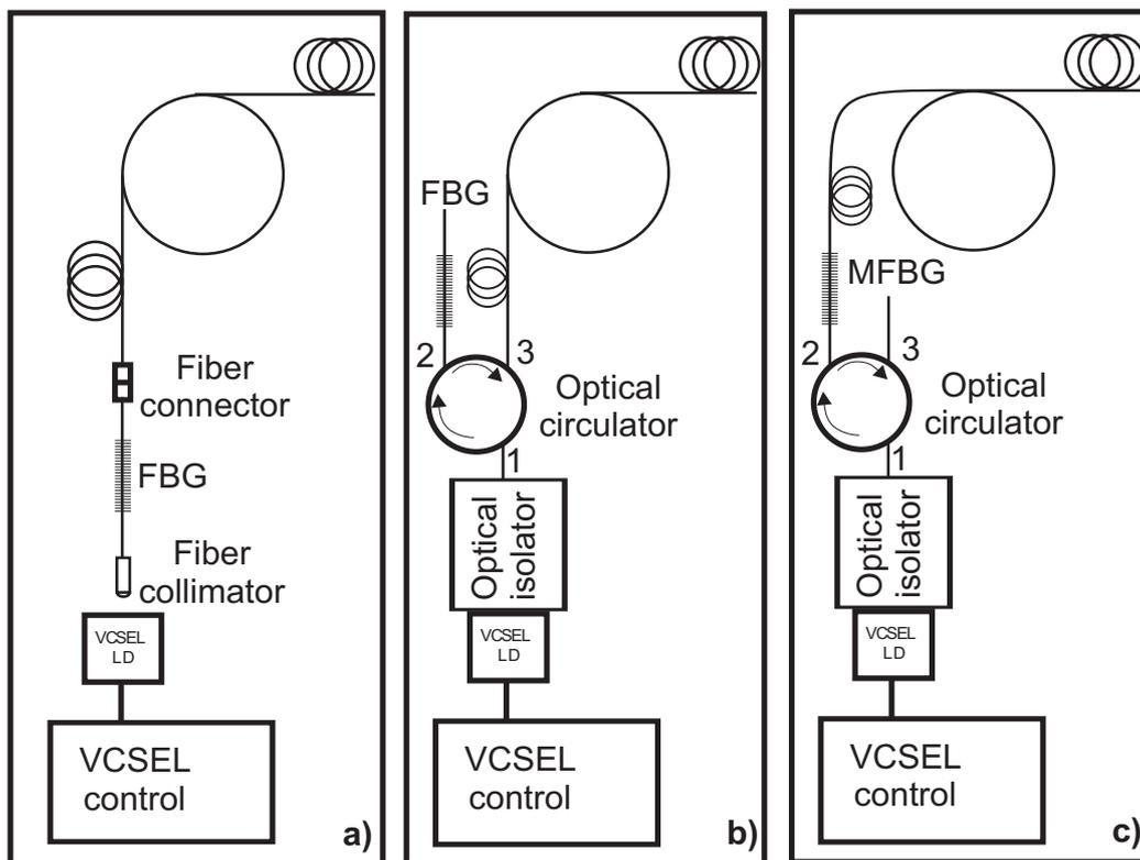
Fig. 10. Improvement of the linewidth of the laser source of the laser interferometer, a) by multiple fiber Bragg grating FBG–FBG is a mirror of an extended cavity of the laser diode, b) by fiber Bragg grating FBG connected by optical circulator– FBG is a frequency filter of the laser diode, c) by multiple fiber Bragg grating MFBG connected by optical circulator – MFBG is a frequency filter of the laser diode.
