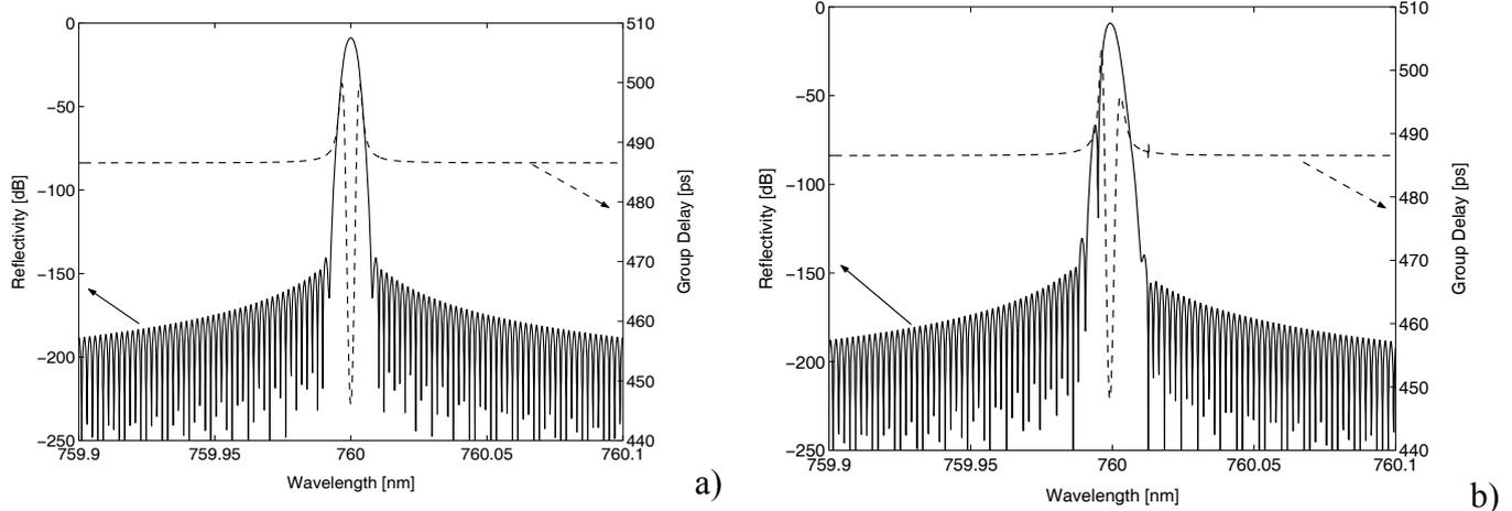
Fig. 5. a) Simulation of reflectivity and group delay spectral characteristics of Gaussian apodized with chirp compensation grating, b) Simulation of reflectivity and group delay spectral characteristics of Gaussian apodized without chirp compensation grating.
