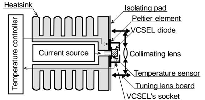
Fig. 2. Configuration of laser head with the VCSEL laser diode
