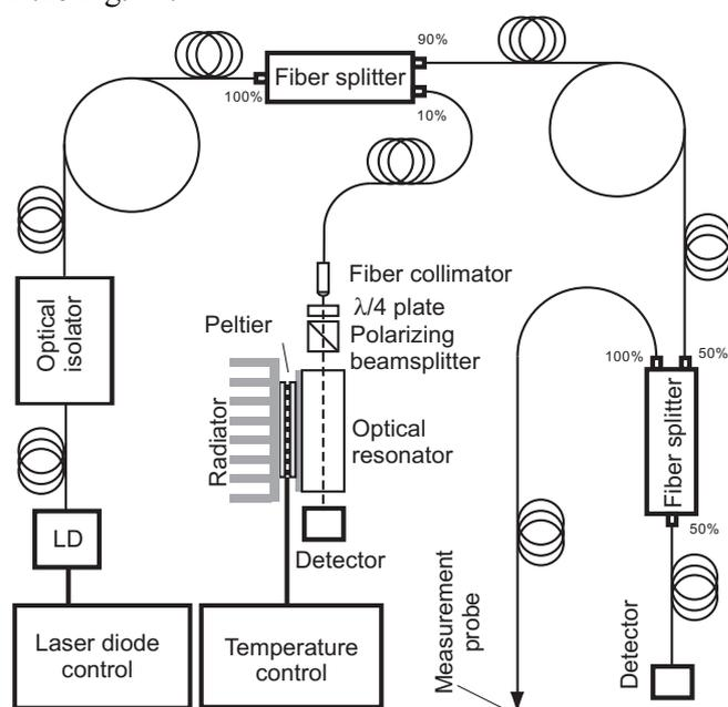
Fig. 9: Set up of the fiber laser interferometer for 760 nm wavelength VCSEL and DFB laser sources.
