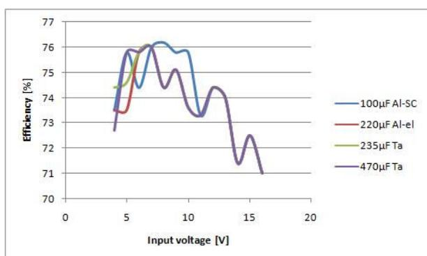
Fig. 19. Efficiency versus input voltage.
