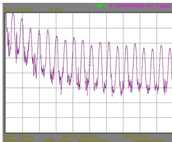
Fig. 15. Frequency spectrum with 100μF in series with 100mΩ.
