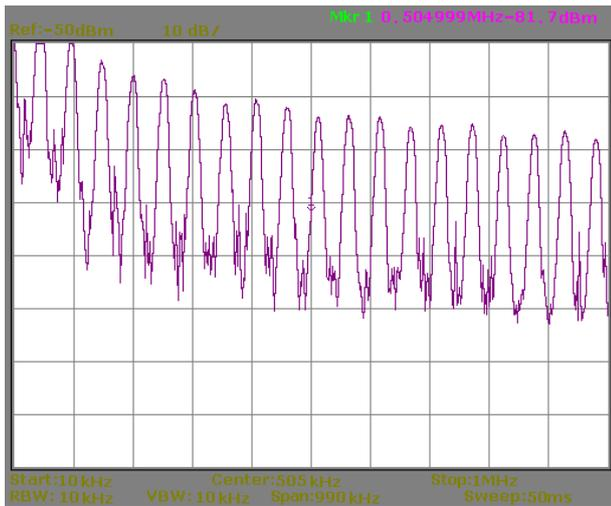
Fig. 17. Frequency spectrum with 100µF in series with 500mΩ.
