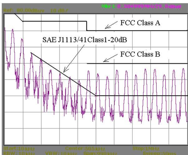
Fig. 10. Frequency spectrum with 100µF SC + 10µF MLCC.
