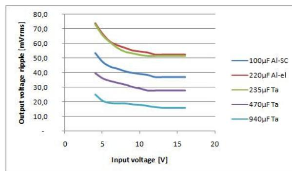
Fig. 20. Output voltage ripple versus input voltage.
