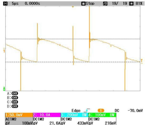
Fig. 6. Output voltage ripple with 220 $\mu\text{F}$  (S.H.I.).
