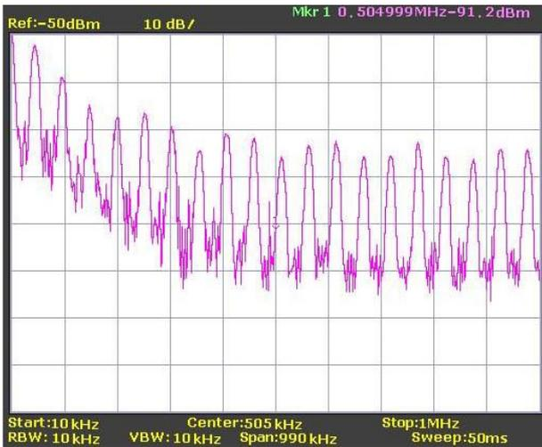
Fig. 8. Frequency spectrum with 100µF Al-SC.
