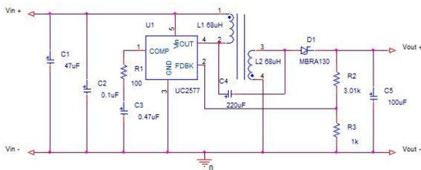
Fig. 4. SEPIC converter with UC2577.
