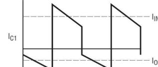
2c. DC coupling capacitor current
