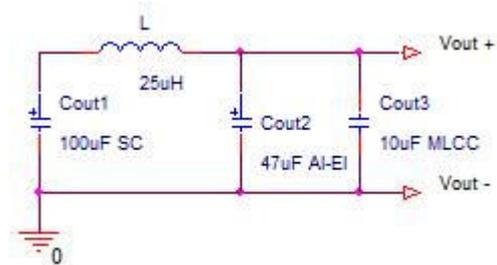
Fig. 12. Output LC Filter added to C<sub>out</sub>.
