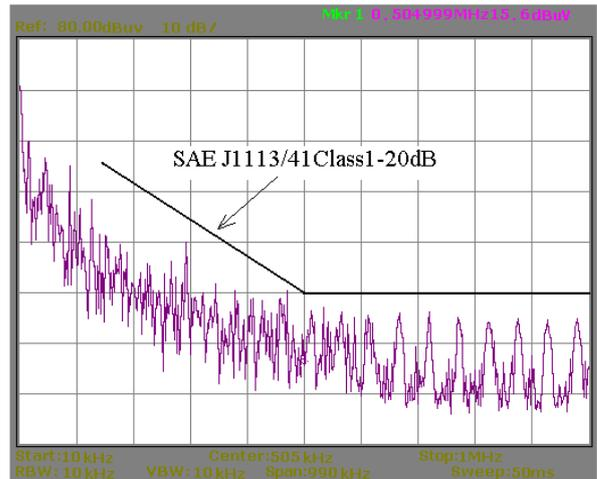
Fig. 11. Frequency spectrum with 100µF Al + 10µF MLCC, and a LC Filter.
