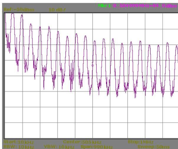
Fig. 16. Frequency spectrum with 100μF in series with 200mΩ.
