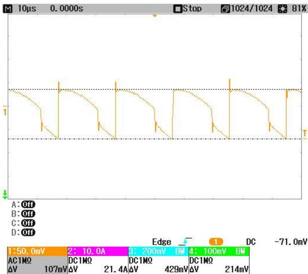
Fig. 5. Output voltage ripple with 100 $\mu\text{F}$  Al-SC.
