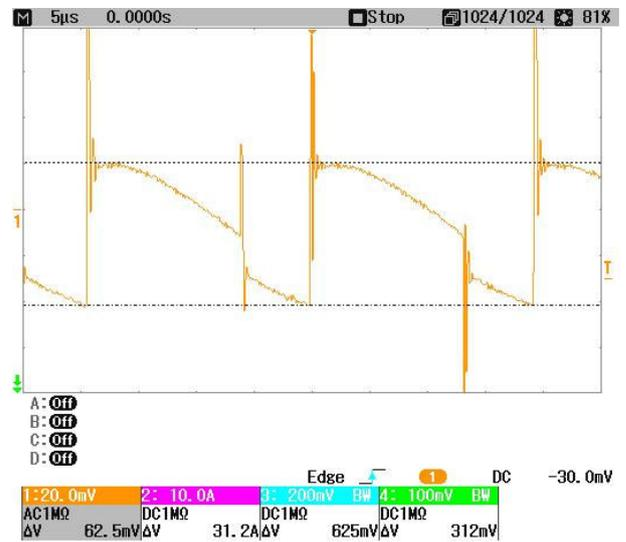
Fig. 7. Output voltage ripple with 470 $\mu\text{F}$  series Ta.
