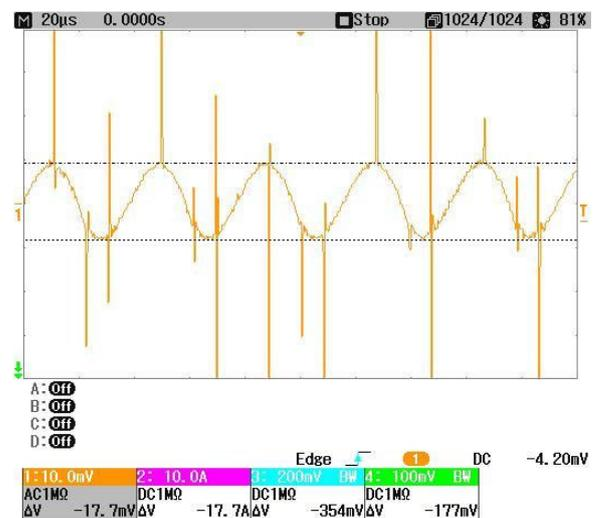
Fig. 13. Output voltage ripple with a LC Filter.
