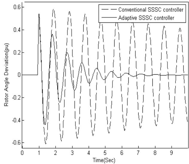
**Fig. 9 Rotor angle response for 3-phase 5-cycle fault**
