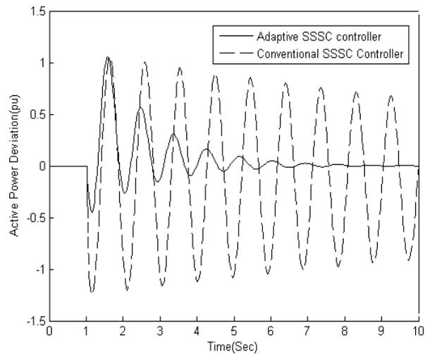
**Fig. 10 Tie-line active power response for 3-phase 5-cycle fault**
