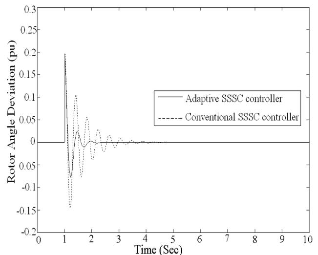
Fig. 3 Rotor angle response for 3-phase 5-cycle fault
