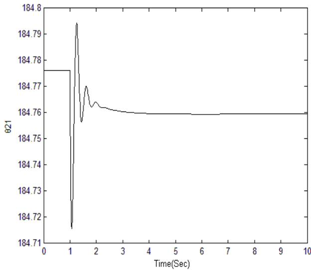
**Fig. 8 The estimated parameter  $\theta_{21}$  response for 3-phase 5-cycle fault**
