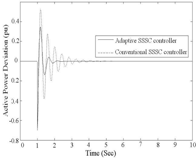
Fig. 4 Tie-line active power response for 3-phase 5-cycle fault
