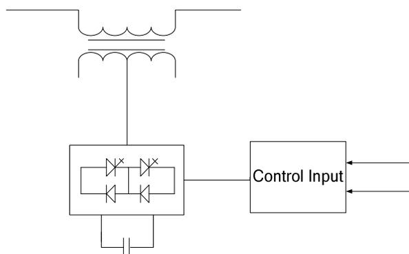
Fig. 1 Schematic diagram of SSSC
