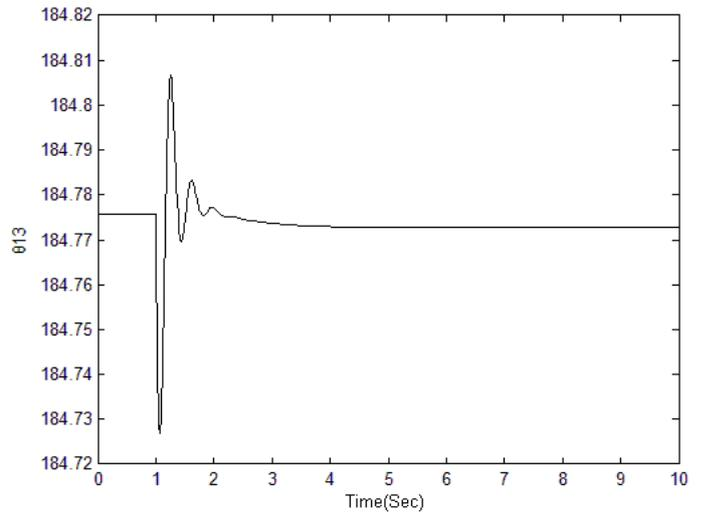
Fig. 7 The estimated parameter  $\theta_{13}$  response for 3-phase 5-cycle fault
