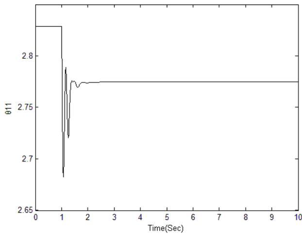
Fig. 5 The estimated parameter  $\theta_{11}$  response for 3-phase 5-cycle fault
