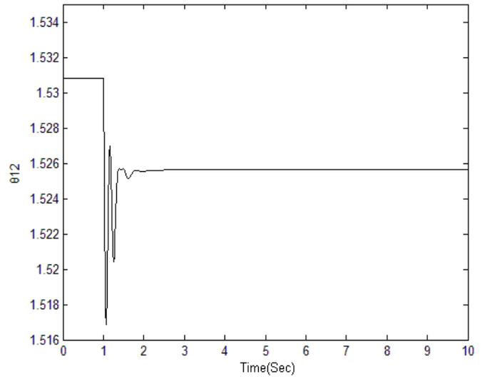
Fig. 6 The estimated parameter  $\theta_{12}$  response for 3-phase 5-cycle fault
