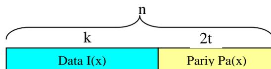
Figure 1: RS encoding
