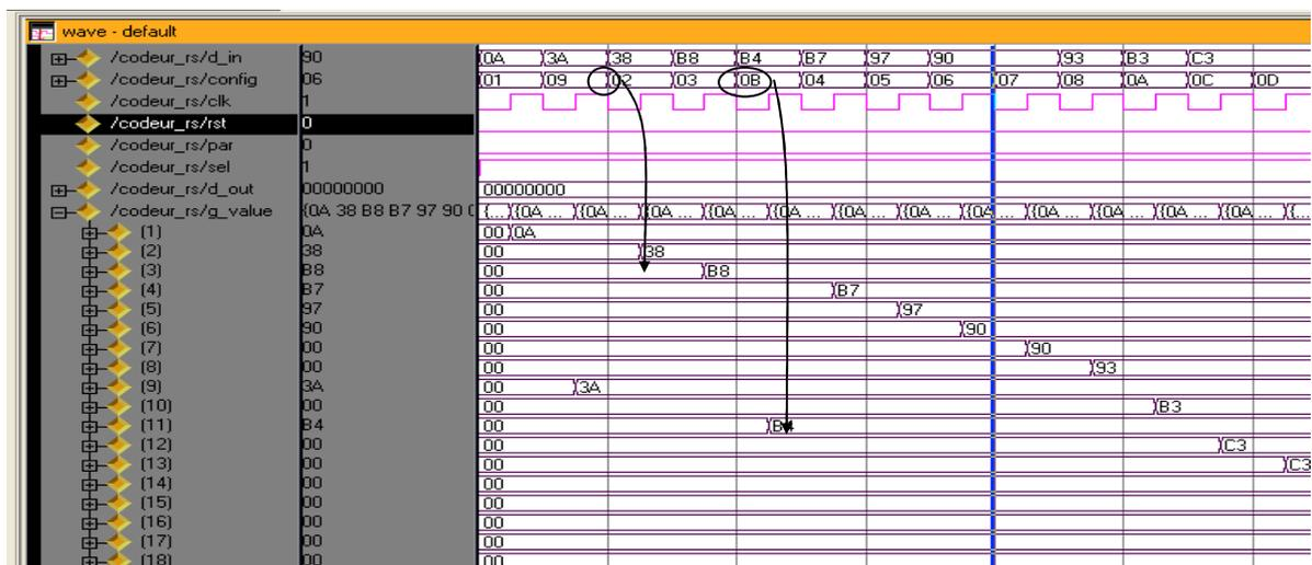
Figure 9b : Configuration step : Downloading a new polynomial
