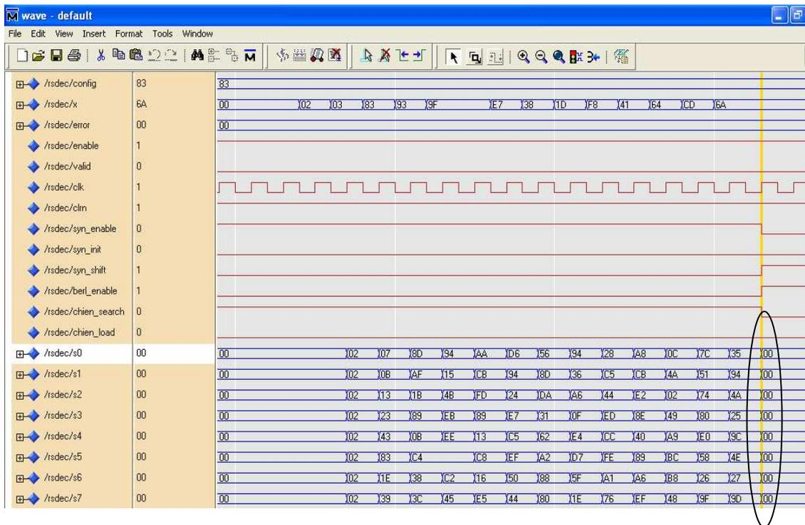
Figure 11 implementation verification of RS (255, 247) decoding (message is received without errors )
