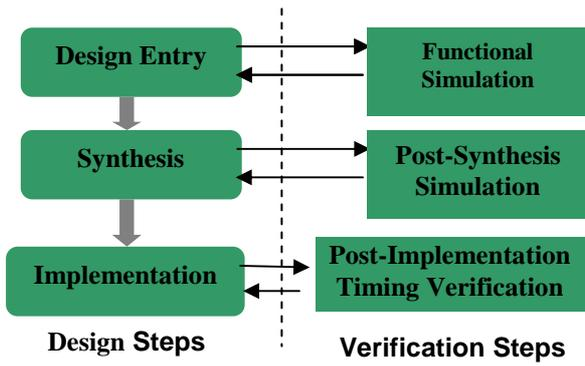
Figure 7: Hardware Verification steps after each design stage [39]
