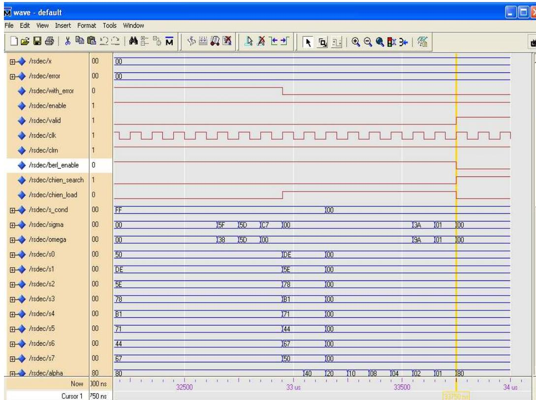
Figure 14 Chien module computing for RS (255, 247) (message is received with errors )
