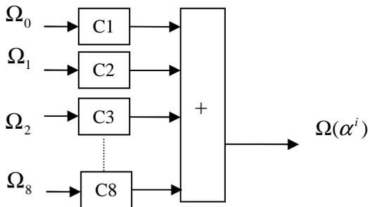
Figure 8  $\Omega(\alpha^i)$  calculator block for  $t = 8$ .
