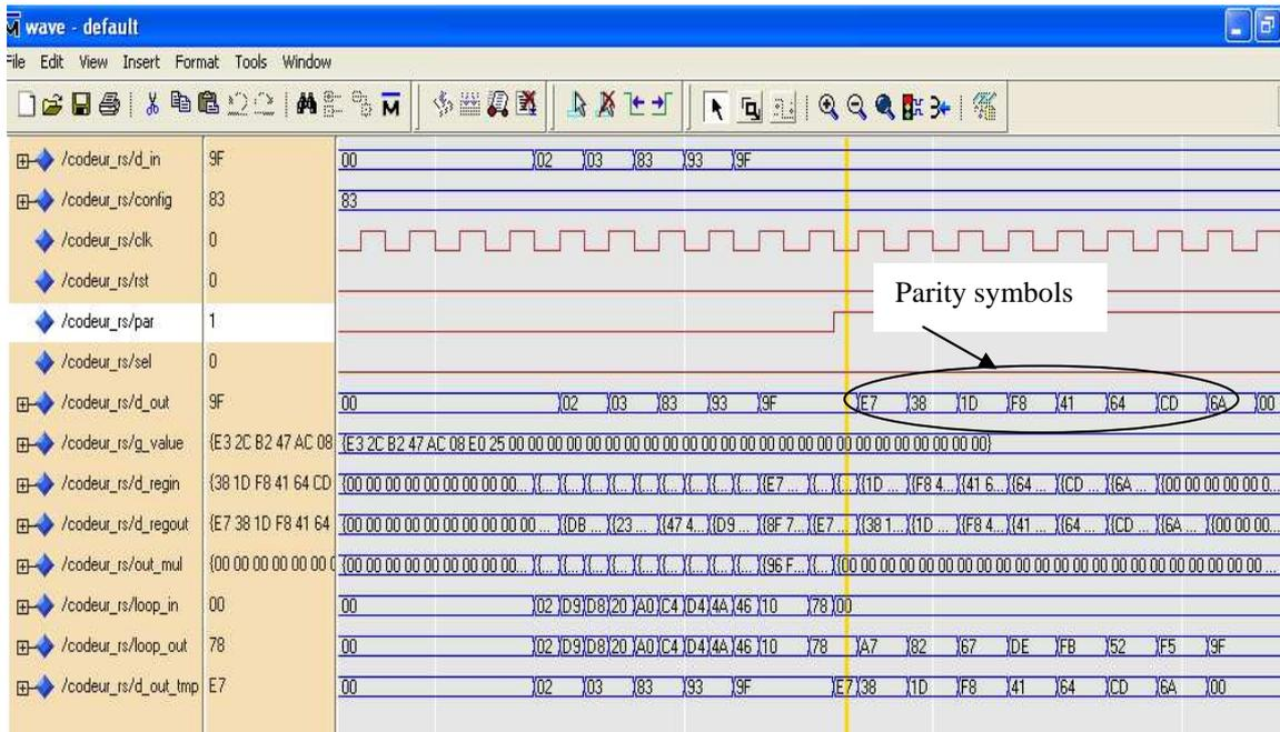
Figure 10: implementation verification of RS (255, 247) encoding
