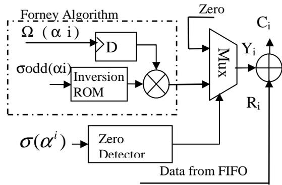
Figure 9 Error value evaluator structure for  $t = 8$ .
