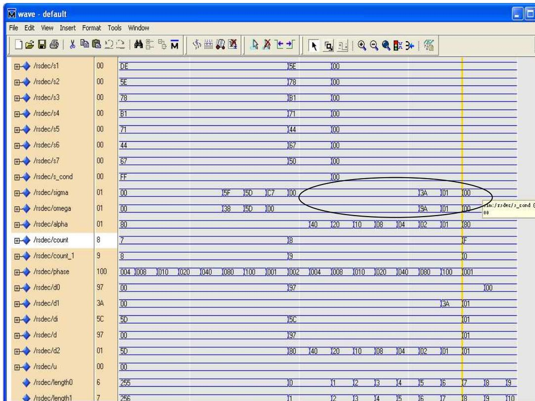
Figure 13 Berlekamp module computing for RS (255, 247) (message is received with errors )
