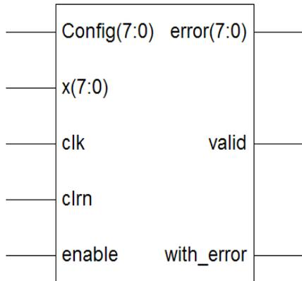
Figure 11 : RS decoder schematic symbol
