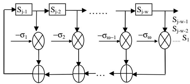
Figure 5 : Berlekamp–Massey algorithm based on LFSR implementation
