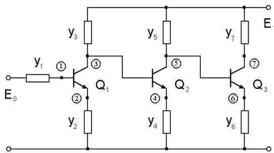
Fig. 7. Three-stage transistor amplifier.
