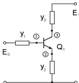
Fig. 5. One-stage transistor amplifier.
