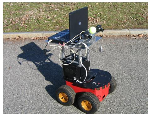
Figure 1: The ActivMedia P2AT rover with stereo head and acquisition PC.
