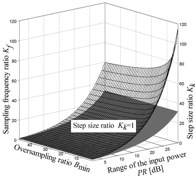
Fig.8. Require adaptation range of step size  $K_k$  (the lower surface) and frequency  $K_f$  (the upper one) versus dynamic range  $DR$  and minimum of  $B_{min}$ .
