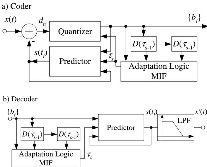
Fig. 2. Block diagram of NS-DM converter; a) coder, b) decoder.
