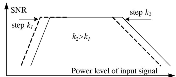
Fig.5. The influence of the step size value  $k$  on the characteristic of SNR vs input level for NS-DM modulation ( $B_{\max}/B_{\min}=\text{const}$ )
