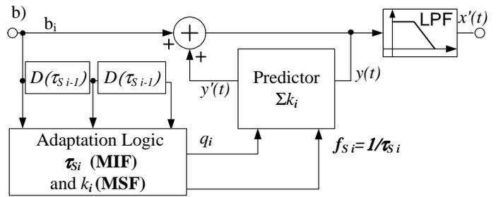
Fig. 4. Block diagram of ANS-DM converter: a) coder, b) decoder.
