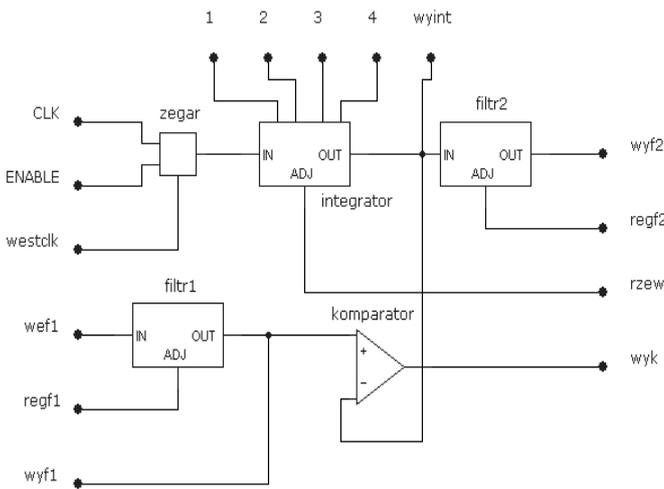
Fig. 9. Diagram of analog NS-DM codec component.
