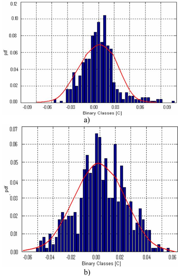
Fig. 9: Histogram and respective Gaussian pdf for random component  $x_{ran_t}$  of  $K_{am}$  (a) and  $K_{av}$  (b). ESI transformer and data from 2005.
