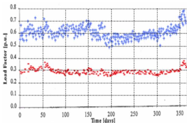
Fig. 7: Annual time series representing daily maximal (denoted with +) and minimal (denoted with -) load factor of distribution transformer ESI. Data from 2005.
