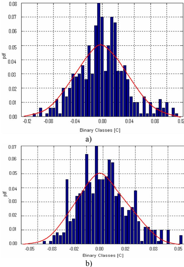
Fig. 8: Histogram and respective Gaussian pdf for random component  $x_{ran_t}$  of  $K_M$  (a) and  $K_m$  (b). ESI transformer and data from 2005.
