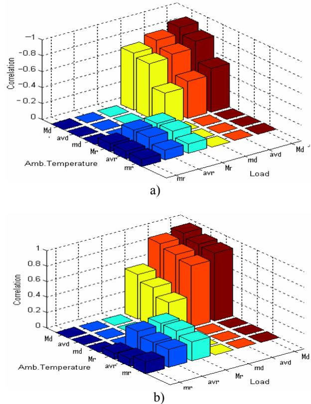
Fig. 13: Deterministic and random correlation between ambient temperature and ESI (a) and BIL (b) profiles. Data from 2004. (Table 6 for ESI transformer).
