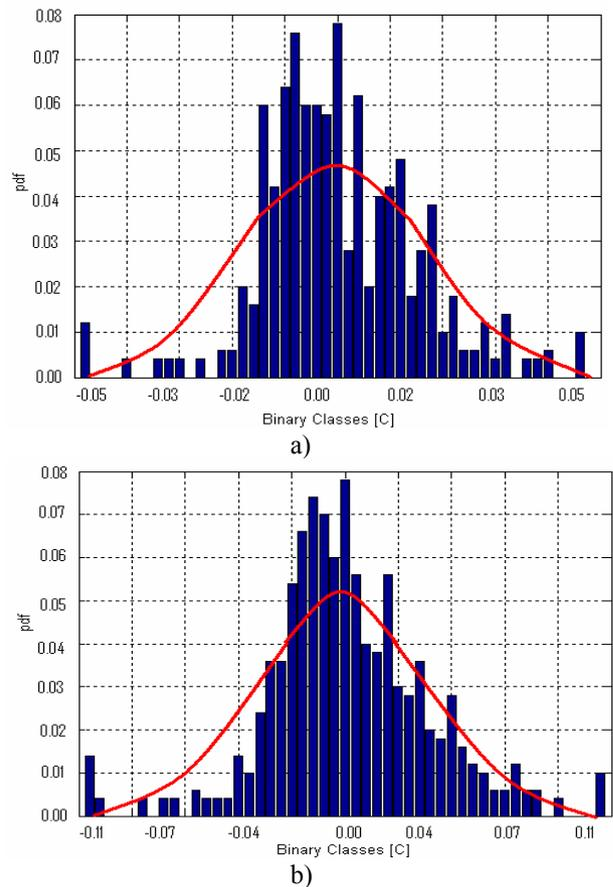
Fig. 10: Histogram and respective Gaussian pdf for random component  $x_{ran}$  of  $K_M$  (a) and  $K_m$  (b). B11 transformer and data from 2004.
