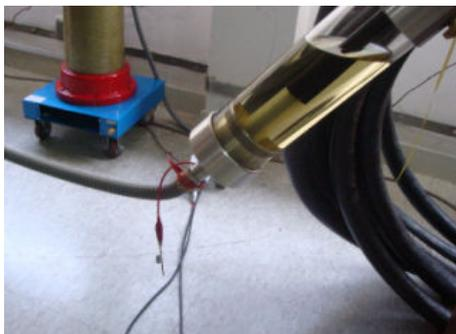
Fig.7 Model of protrusion on high voltage conductor.
