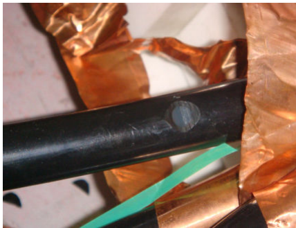
Fig.8 Model of scratch on cable extern shielding tier
