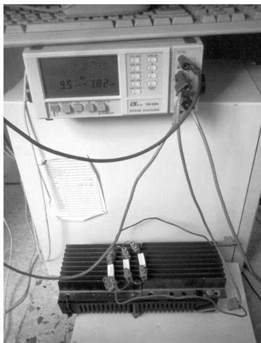
Fig. 9 Experiment system with resistive load
