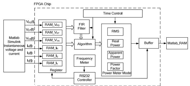
Fig. 5. Systematic structure diagram of calculation.
