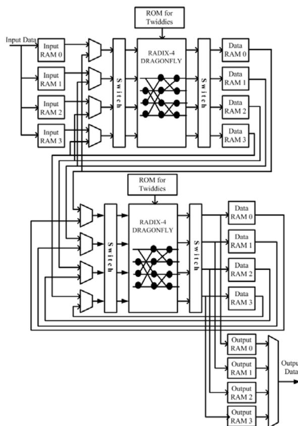
Fig. A1. Structure diagram of radix-4 FFT core.
