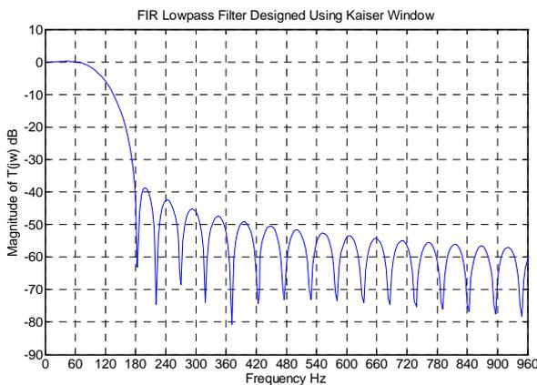
Fig.2. Low-pass filter designed by Kaiser window.
