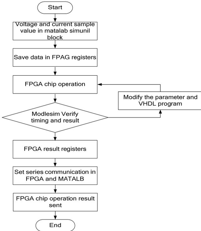
Fig. 6. The flowchart of FPGA design circuit.
