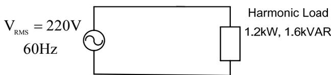
Fig.3. Single-phase circuit including harmonic current sources.
