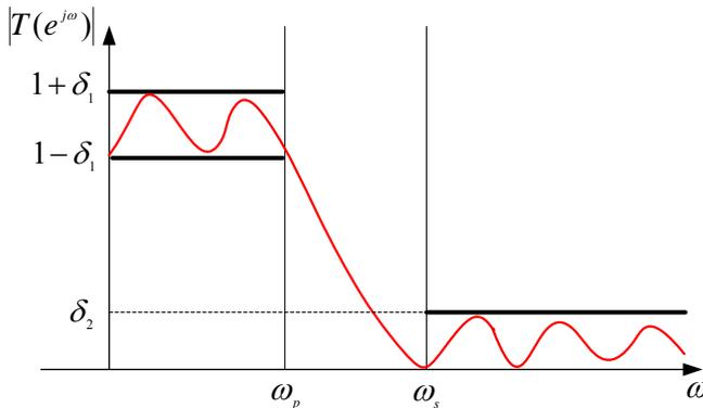
Fig. 1. Band characteristics of a low-pass filter.
