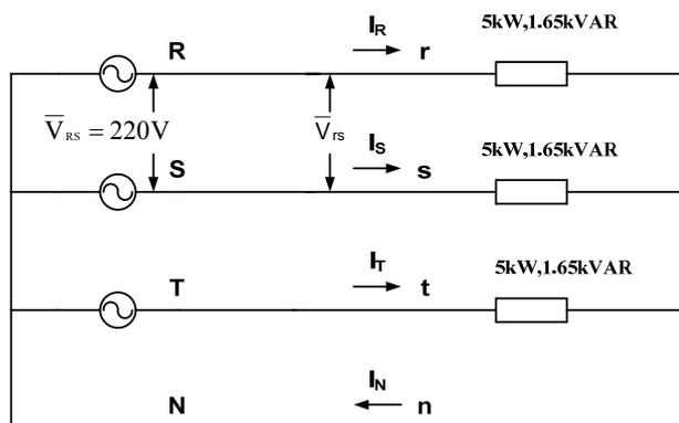
Fig. 4. Three-phase four-wire simulation system
