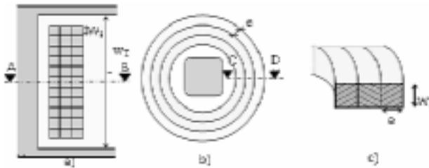
Fig. 9: (a) longitudinal section of transformer winding (one side) showing 3 layers and 11 turns per layer (b) view AB; cross section of transformer winding turn with 3 layers (conductors) (c) view CD; winding turn cross-section with 3 layers (conductors)
