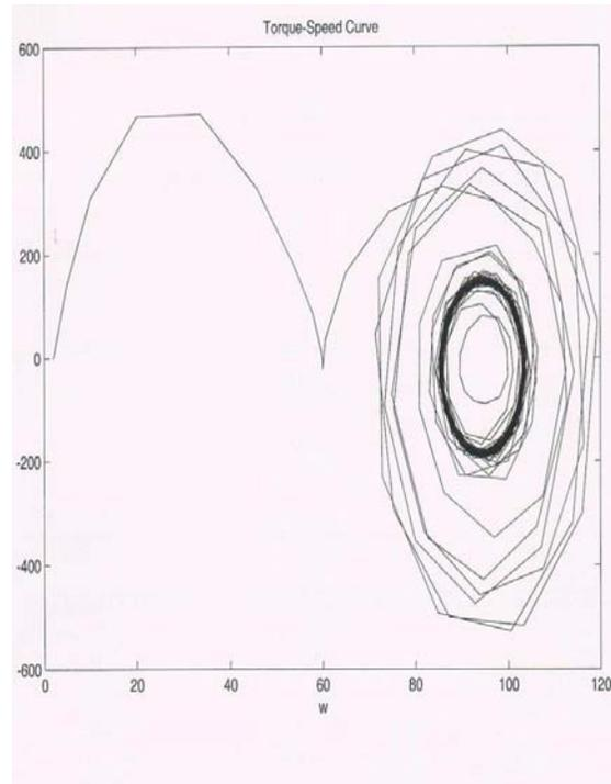
Fig.4 Curve of torque-speed for  $K=10$ ,  $r_{ex}=0.016$ ,  $V_{wind}=4$ ,  $\Theta=-0.78$ ,  $N_g=15$ .
