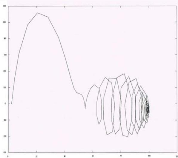
Fig.3 Curve of torque-speed for  $K=15$ ,  $r_{ex}=3$ ,  $V_{wind}=5$ ,  $\Theta=-0.78$ ,  $N_g=12$ .
