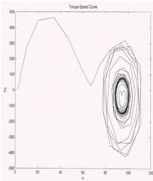
Fig.2 Curve of torque-speed for  $K=15$ ,  $r_{ex}=0.016$ ,  $V_{wind}=5$ ,  $\Theta=-0.78$ ,  $N_g=12$ .
