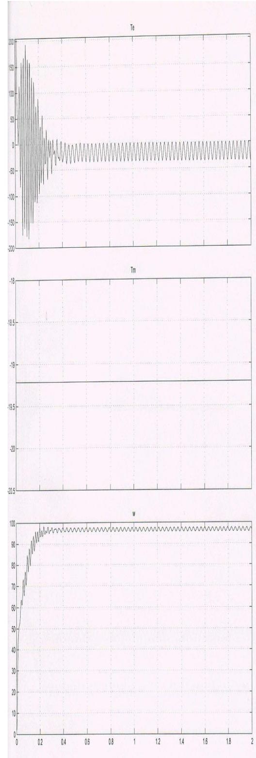
Fig.9 Curve of torques and mechanical rotor speed for  $K=10$ ,  $r_{ex}=3$ ,  $V_{wind}=4$ ,  $\Theta=-0.78$ ,  $N_g=15$ .
