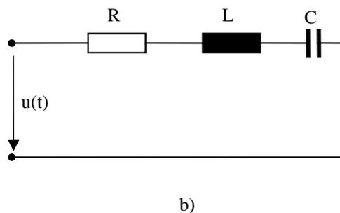
Fig.2 a) Mechanical system with a single degree of freedom; b) RLC series circuit
