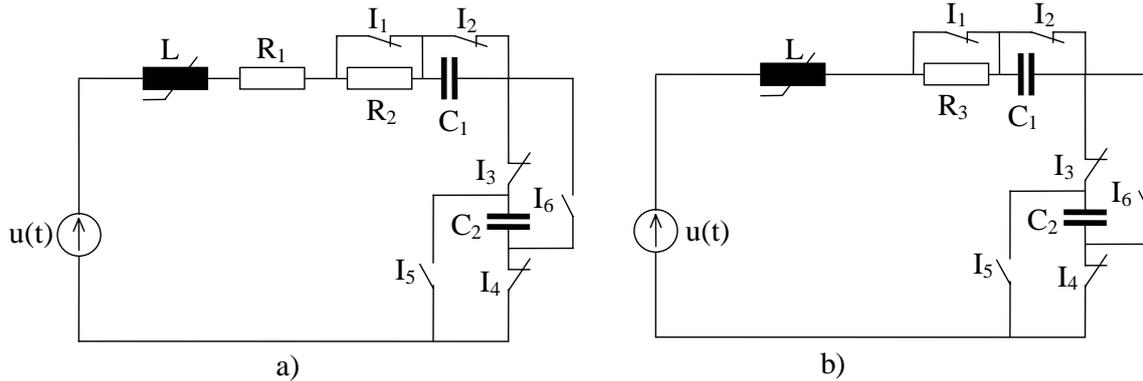
Fig.5 Electrical circuits for simulation of mechanical system for closing operation a), for opening operation b)
