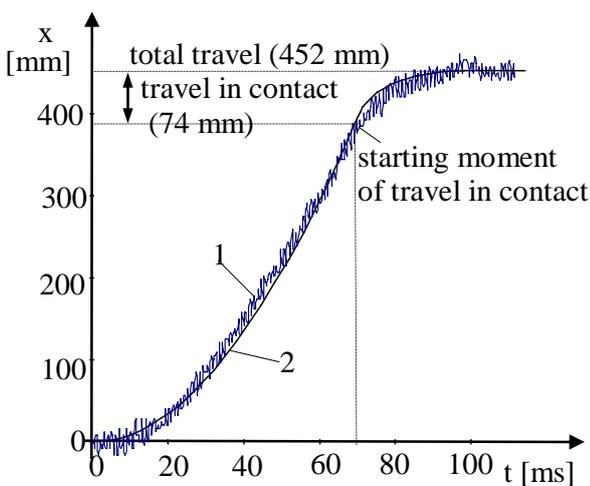
Fig.6 Travel of movable rod during the closing operation experimental (curve 1) and numeric (curve 2) determined, respectively
