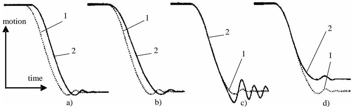
Fig.1 The motion of movable contact at disconnection in normal situation (1), abnormal respectively (2)
