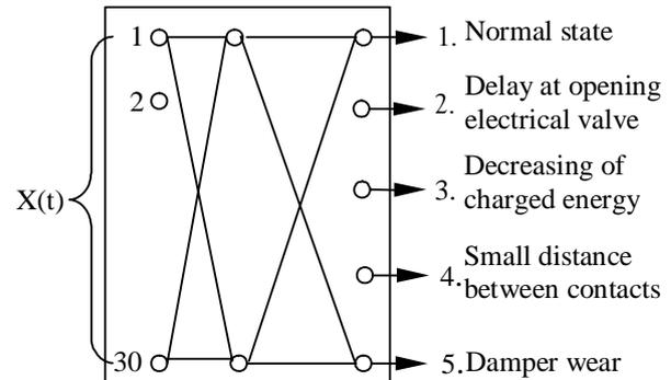
Fig.8 ANN architecture for the monitoring of kinematics characteristics
