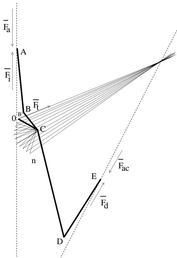
Fig.4 The forces which acting to kinematics chain of circuit breaker
