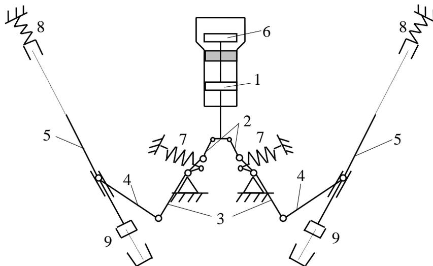
Fig.3 Mechanical system of a HV circuit breaker
