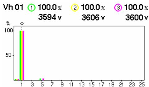
Fig.11. Harmonic spectra of the phase voltages at the end of the melting process
