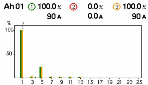
Fig.13. Harmonic spectra of the currents at the end of the melting process
