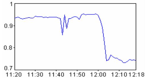
Fig.16. Recorded values of PF per phase 1 in the cold state
