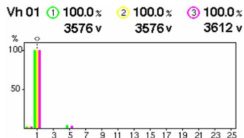
Fig.3. Harmonic spectra of the voltages in the cold state of the charge
