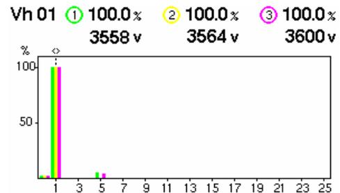
Fig.7. Harmonic spectra of the voltages in the intermediate state
