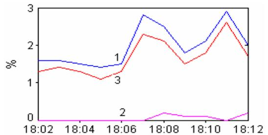
Fig.22. Recorded values of  $V_{THD}$  in the last stage of the melting process
