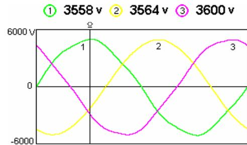
Fig.6. Phase voltages in the intermediate state
