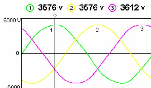
Fig.2. Phase voltages in the cold state of the charge
