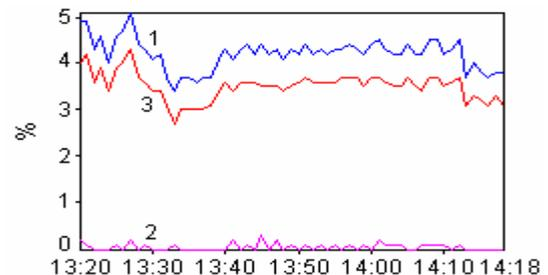
Fig.18. Recorded values of  $V_{THD}$  in the intermediate state
