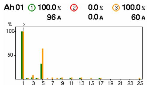
Fig.9. Harmonic spectra of the currents in the intermediate state
