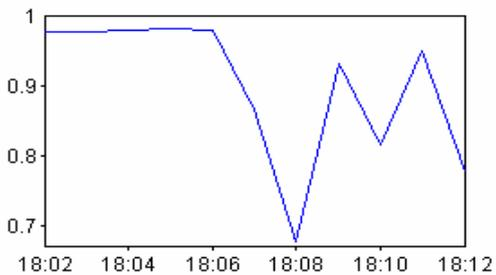
Fig.24. Recorded values of PF per phase 1 in the last stage of the melting process
