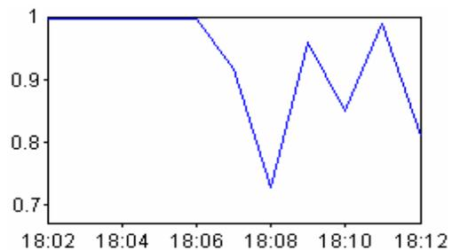
Fig.25. Recorded values of DPF per phase 1 in the last stage of the melting process
