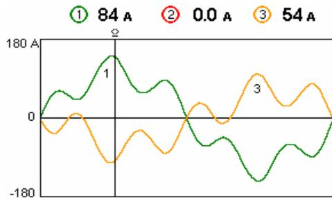
Fig.4. Line currents in the cold state of the charge
