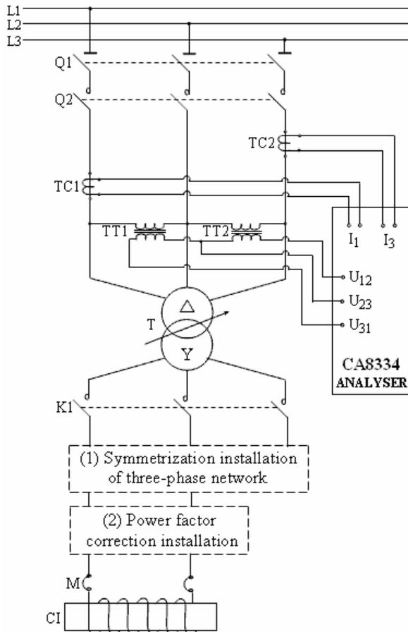
Fig.1. Experimental electric diagram
