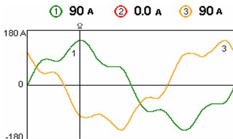
Fig.12. Line currents at the end of the melting process
