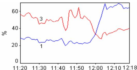
Fig.15. Recorded values of  $I_{THD}$  in the cold state
