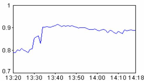
Fig.20. Recorded values of PF per phase 1 in the intermediate state
