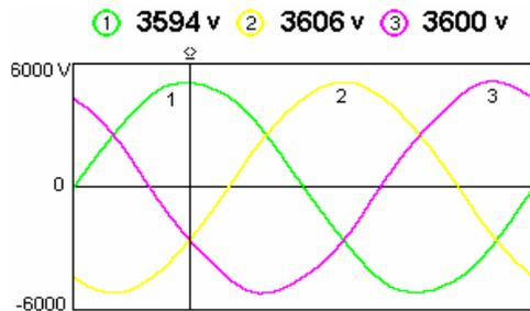
Fig.10. Phase voltages at the end of the melting process
