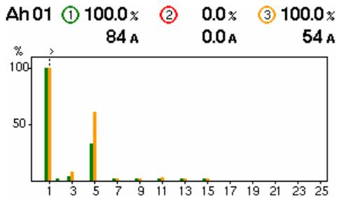
Fig.5. Harmonic spectra of the currents in the cold state of the charge
