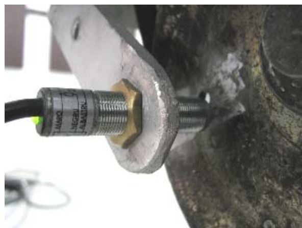
Fig.8. Mounting of the speed transducer
