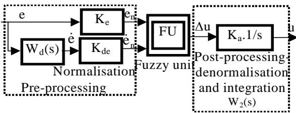
Fig.4. Incremental PI Fuzzy Logic Controller
