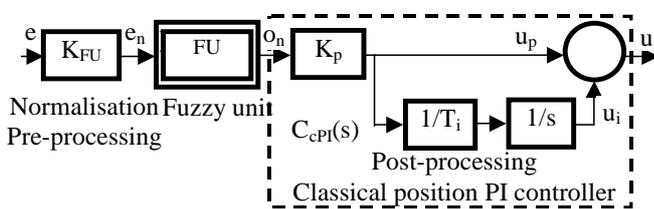
Fig.3. Position PI Single Input Fuzzy Controller
