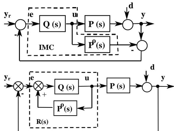
Fig.11. Block diagram of system with IMC – original and after equivalent transformation
