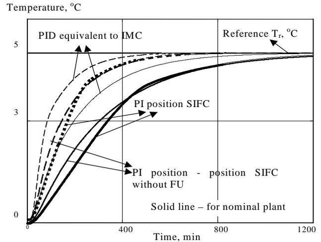
Fig.13. Step responses of systems with PI position SI FC, PI position – position SIFC without FU and PID equivalent to IMC
