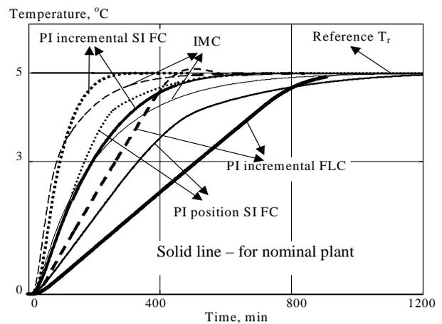
Fig.10. Step responses of PI incremental FLC, PI incremental SI FC, PI position SI FC and IMC systems
