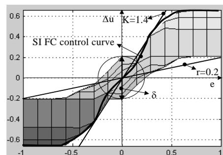
Fig.8.  $e-\Delta u$  projection of FU control surface of FLC
