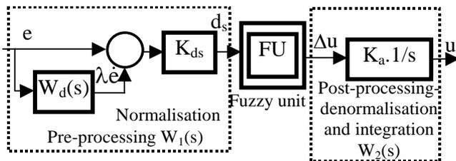
Fig.2. Incremental PI Single Input Fuzzy Controller
