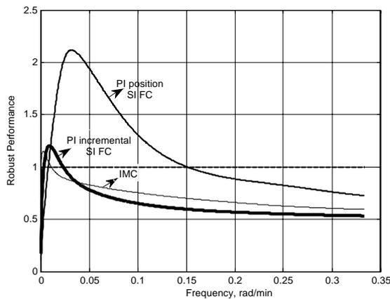
Fig.12. Robust performance curves of PI incremental SI FC, PI position SI FC and IMC systems
