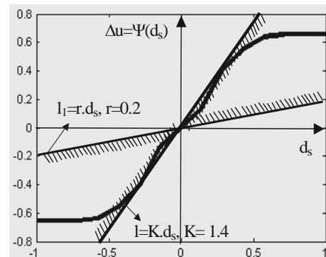
Fig.5. Sector bounded static FU nonlinearity
