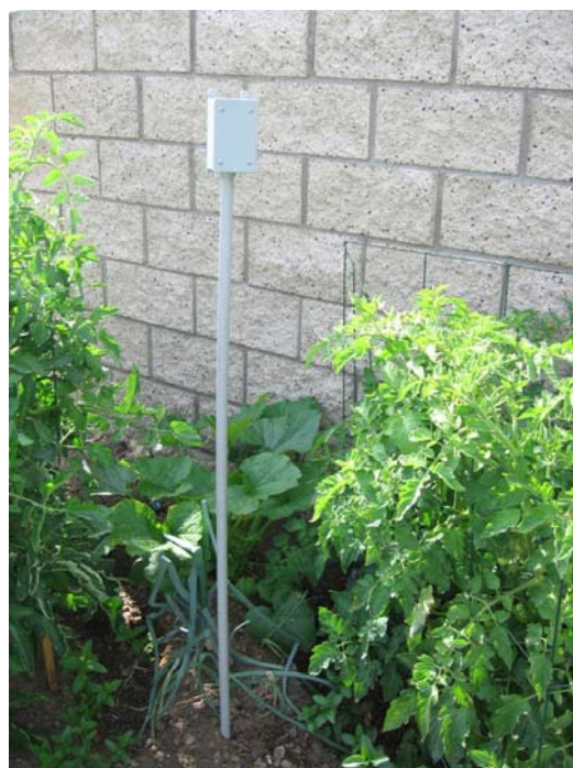
Fig. 2: WSN unit with microprocessor, transmitter, battery and built-in sensors for monitoring atmospheric temperature and humidity and wired sensors for wind speed/ direction and
