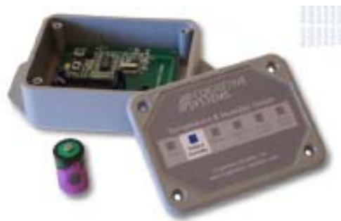
Fig. 2: WSN unit with microprocessor, transmitter, battery and built-in sensors for monitoring atmospheric temperature and humidity and wired sensors for wind speed/ direction and
