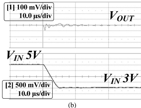
Fig. 9. Line transient response: Input voltage  $V_{IN}$  changes (a) from 3V to 5V (b) from 5V to 3V.
