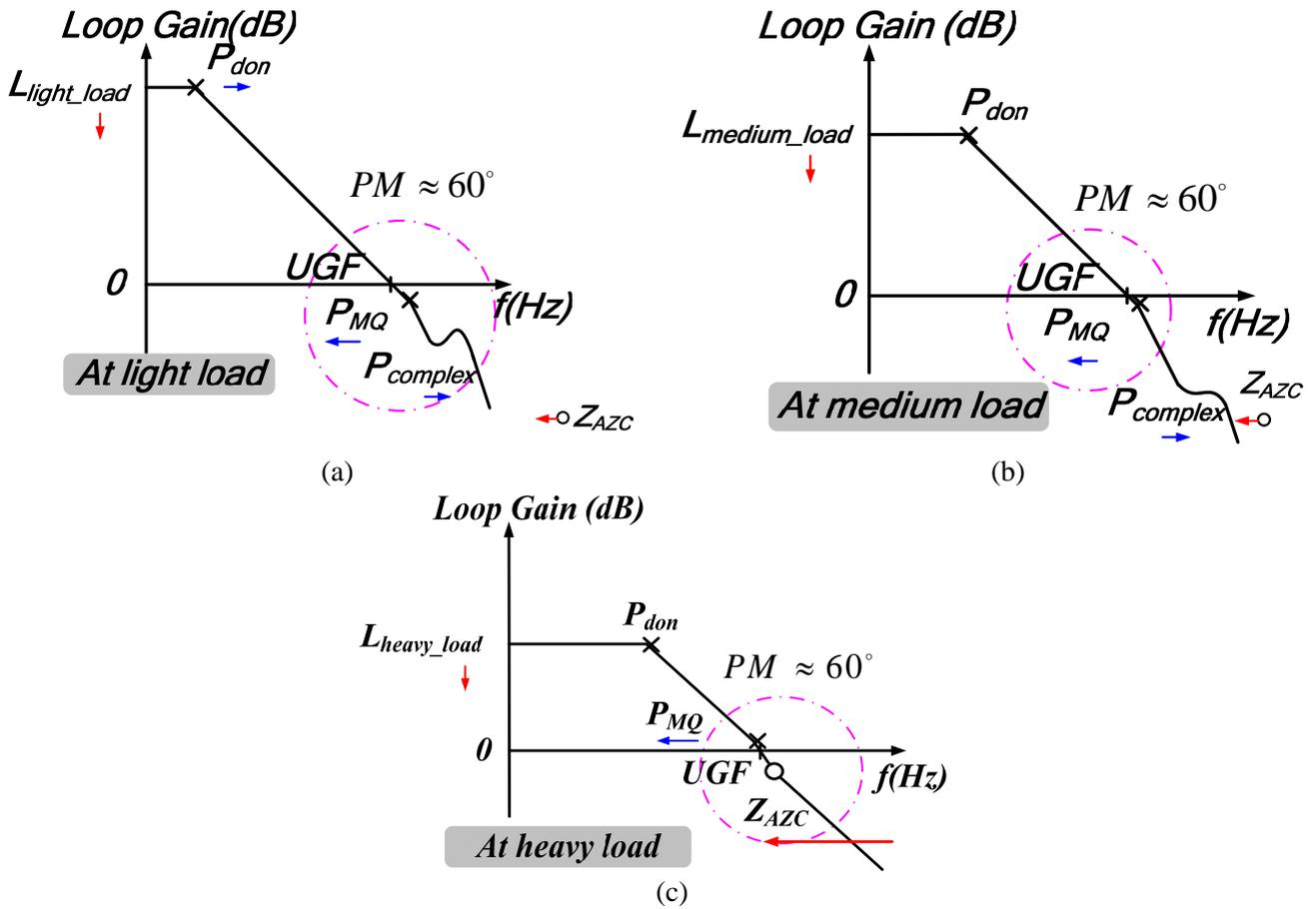
Fig. 4. The locations of poles and zero at different loads. (a) Poles and zero at ultra light loads. (b) Poles and zero at medium loads. (c) Poles and zero at heavy loads.
