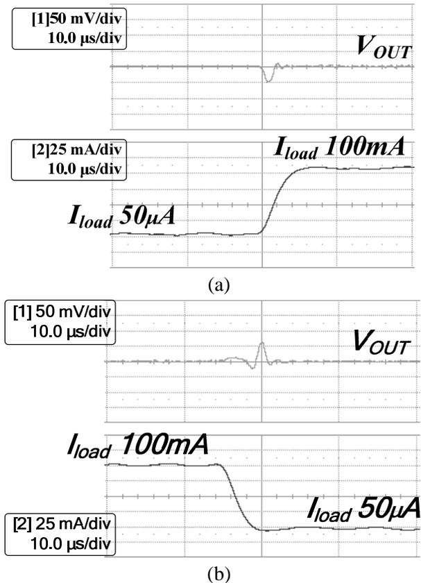
Fig. 8. Load transient response: Load current  $I_{load}$  changes (a) from 50 $\mu$ A to 100mA (b) from 100mA to 50 $\mu$ A.
