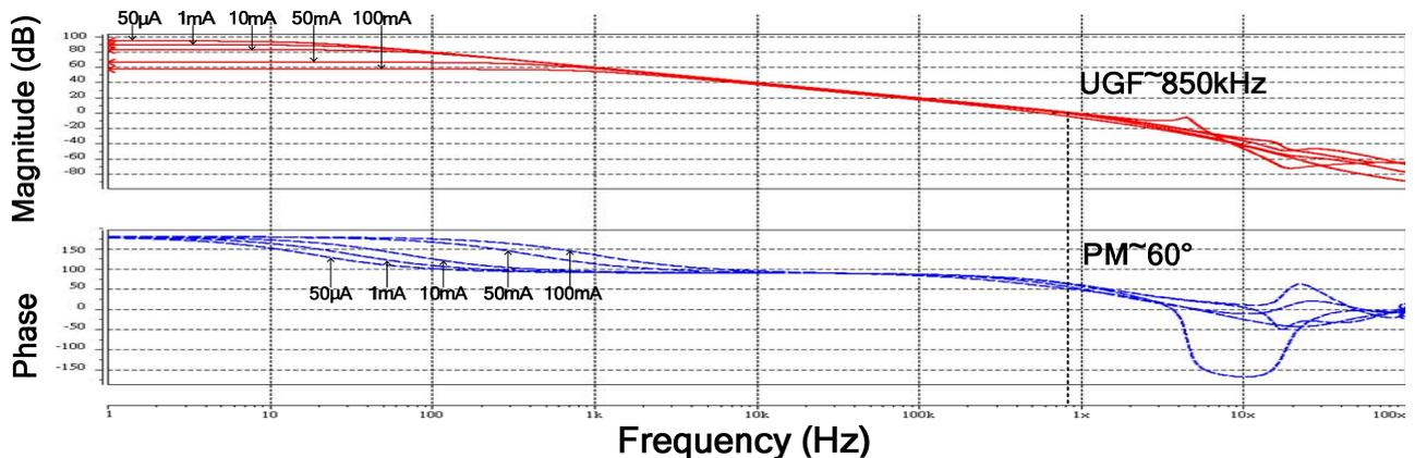
Fig. 6. Frequency response of loop gain at different loads.
