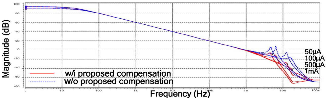
Fig. 7. The frequency peaking with and without the MQ compensation at different light loads.
