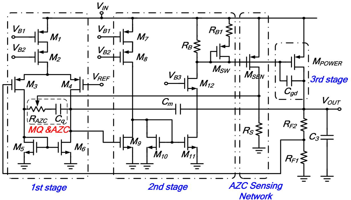
Fig. 5. The schematic of capacitor-free LDO regulator with the MQ and AZC techniques.
