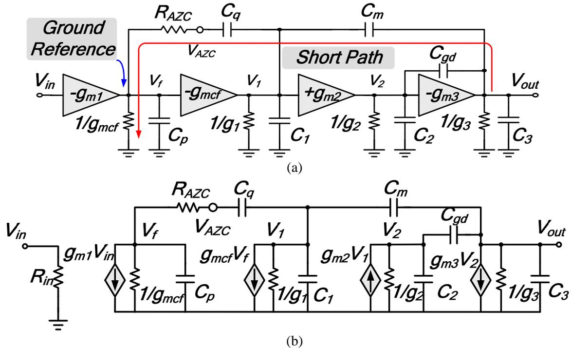
Fig. 3. Topology of capacitor-free LDO regulator with MQ and AZC technique. (a) Structure of the proposed circuit. (b) Small-signal of the proposed circuit.
