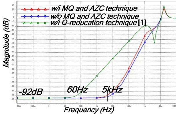
Fig. 10. PSR performance for different compensation techniques at load current  $I_{load}=1mA$ .
