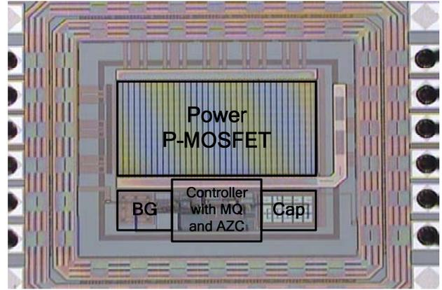
Fig. 11. Chip micrograph.
