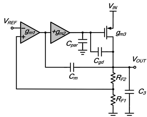
Fig. 1. Conventional three-stage capacitor-free LDO regulator.
