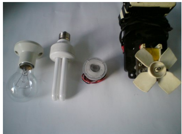
Fig. 7 A.C. loads; incandescent lamp, CFL, power LED and induction motor
