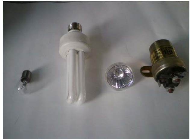
Fig. 6 D.C. loads; incandescent lamp, CFL, halogen lamp and permanent magnet D.C. motor
