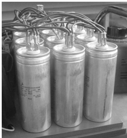
Fig 3c: discharging capacitor block
