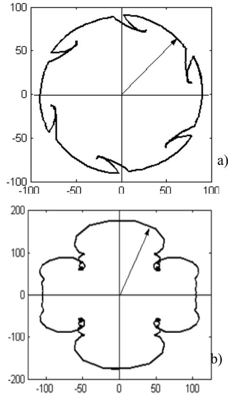
Fig. 1 Geometric place of the voltage space vector modulus: to input of a three-phase bridge controlled rectifier - a) and to output of a voltage inverter - b)
