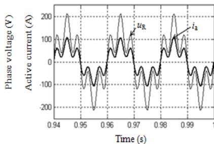
Fig. 18 Akagi's active current related to supply voltage in the case of linear balanced load
