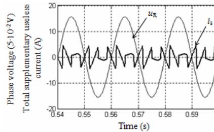
Fig. 12 Phase voltage and total supplementary useless current
