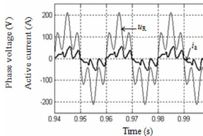
Fig. 21 Akagi's active current related to supply voltage in the case of nonlinear balanced load
