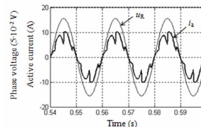
Fig. 8 Phase voltage and active current defined by Akagi
