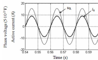
Fig. 7 Phase voltage and proposed active current waveforms
