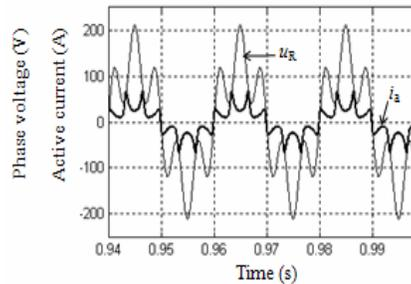
Fig. 20 Nonsinusoidal supply voltage and active current, as defined by (8), in the case of nonlinear balanced load
