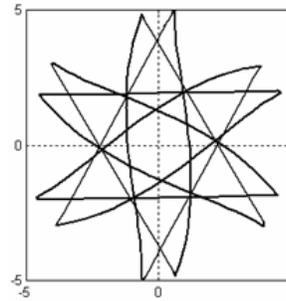
Fig. 13 Space-vector trajectory of the supplementary useless current
