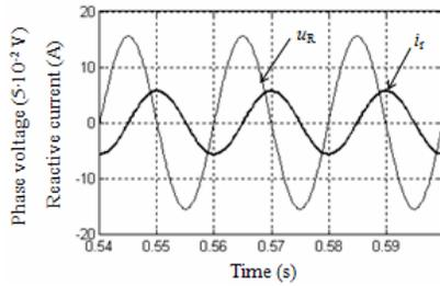
Fig. 9 Phase voltage and proposed reactive current waveforms
