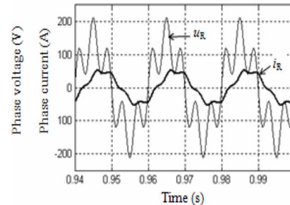
Fig. 19 Nonsinusoidal supply voltage and current waveforms in the case of RL load
