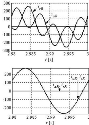
Fig. 5 The Akagi's current components and identical current components of CPC's and proposed theories in line R
