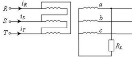
Fig. 2 - Three-phase circuit with single-phase purely resistive load
