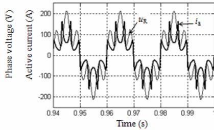
Fig. 15 Nonsinusoidal supply voltage and active current, as defined by (8), in the 5.5 case
