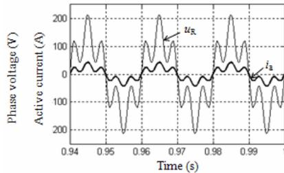
Fig. 23 Nonsinusoidal supply voltage and active current, as defined by (22), in the case of nonlinear balanced load
