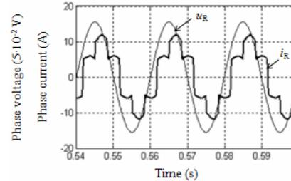
Fig. 6 Phase voltage and current in the primary of the transformer
