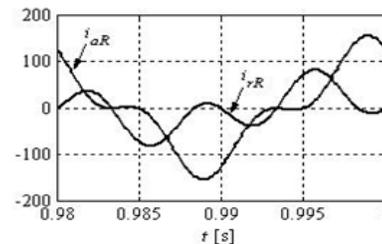
Fig. 3 The Akagi's current components in line R
