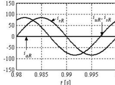
Fig. 4 The identical current components of CPC's and proposed theories in line R for purely inductive load
