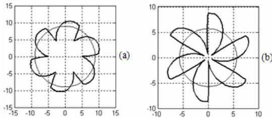
Fig. 11 Space-vector trajectories of the active current (a) and reactive current (b) defined by Akagi (thin line) and proposed (thick line) by (8) and (9)
