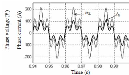
Fig. 14 Nonsinusoidal supply voltage and current waveforms in the case of purely resistive load
