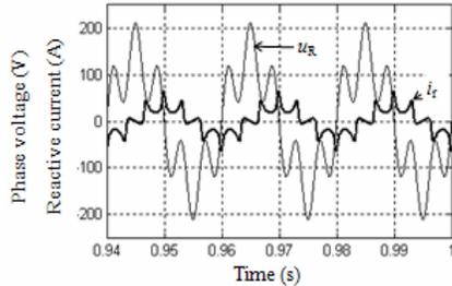
Fig. 22 Nonsinusoidal supply voltage and reactive current, as defined by (9), in the case of nonlinear balanced load
