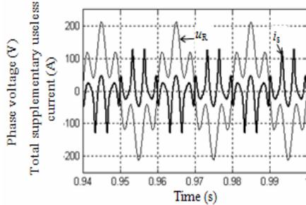
Fig. 17 Total supplementary useless current, as defined by (12), related to supply voltage in the case of linear balanced load
