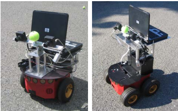
Figure 2: The Pioneer 3DX (left) and 2AT (right) rovers, equipped with stereo head and controlling PC.
