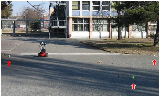
Figure 4: The Pioneer 2AT rover on the test field. Red arrows indicate the measurement base targets.
