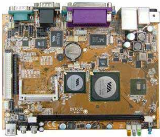
Fig. 2 CV 700C motherboard
