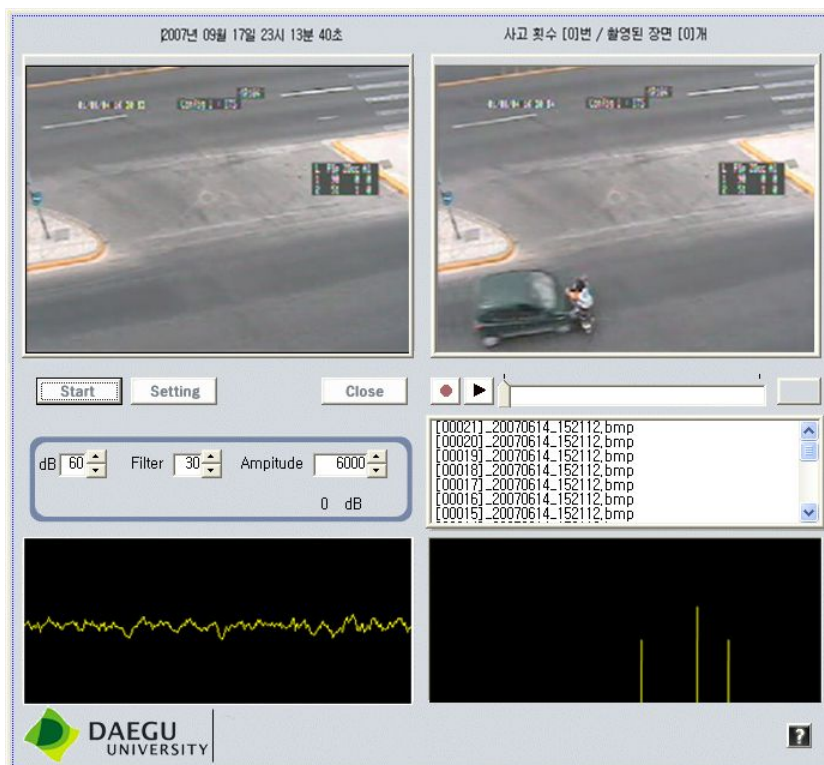
Fig. 9. The application program. (First row: screen shots before and after an accident, Second row: sound and frequency environment setting, Third row: a normal signal and frequency spectrum of an accident signal).
