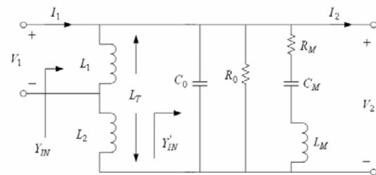
Fig. 6 Equivalent circuit of Tonpiltz transducer with matching transformer.
