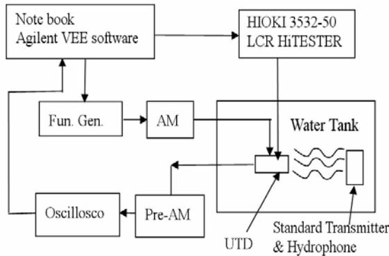
Fig. 7 Diagram of PC\_base Measurement System.
