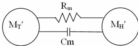
Fig. 2 Simple spring-mass model of Tonpiltz Transducer.
