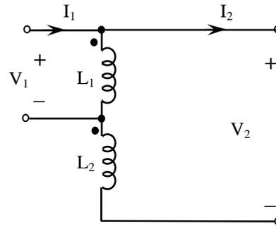
Fig. 9 Self-coupling transformer.
