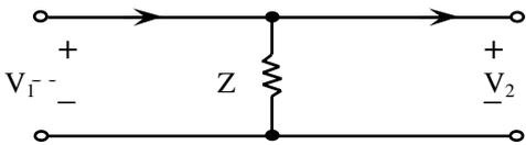
Fig. 8 Circuit with shunt impedance.
