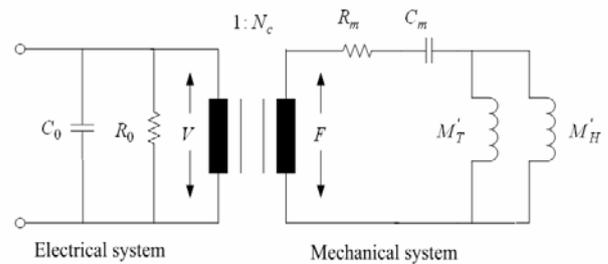
Fig. 3 Equivalent circuit of Tonpiltz transducer working in air.
