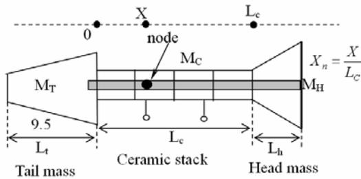
Fig. 1 Tonpiltz transducer cross-section
