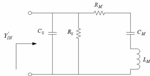
Fig. 4 Simplified equivalent circuit of Tonpiltz transducer.
