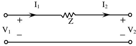
Fig. 7 Circuit with serial impedance.
