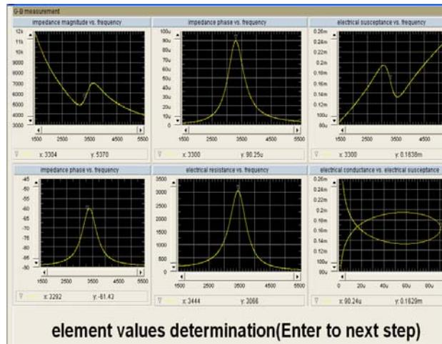
Fig. 10 G-B measurement for unmatching Transducer.
