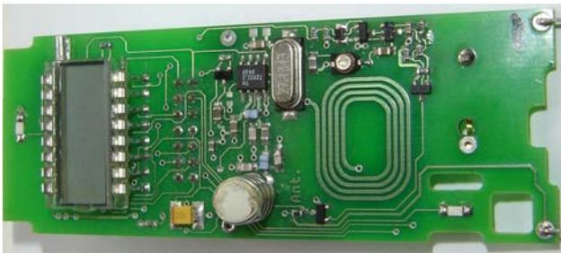
Figure 11 - MSP430F417 based sensor with transmitter
