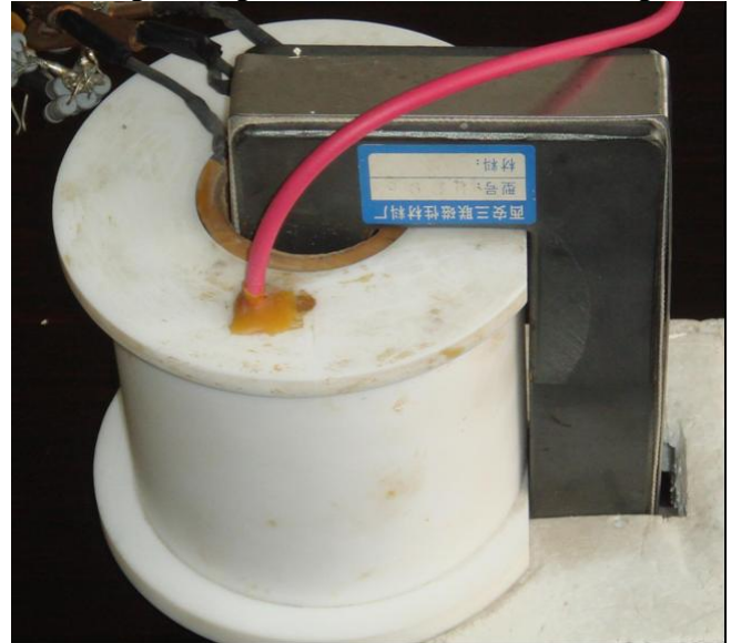
a. The overall picture of the HF high voltage transformer
