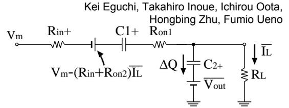
Fig.7 Instantaneous equivalent circuit in *State - T1*.
