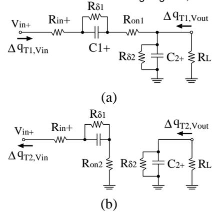
Fig.4 Instantaneous equivalent circuits of converter block-1. (a) *State - T1*. (b) *State - T2*.
