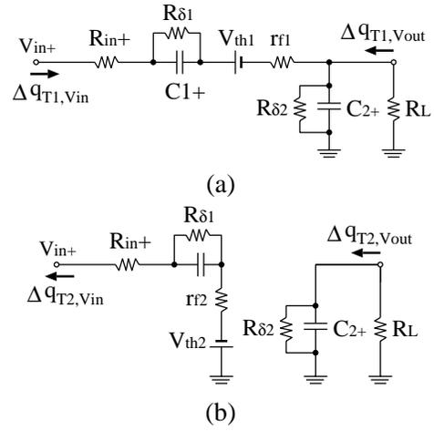
Fig.12 Instantaneous equivalent circuits of the conventional converter block. (a) *State - T1*. (b) *State - T2*.
