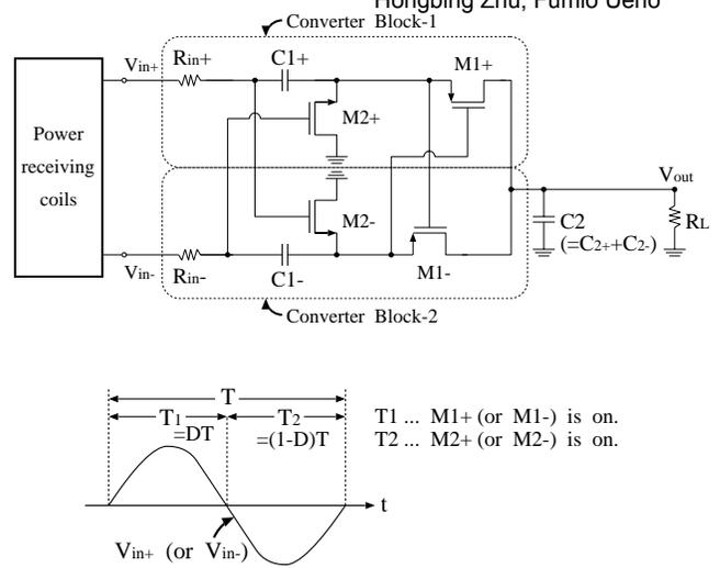
Fig.3 Proposed AC-DC converter.
