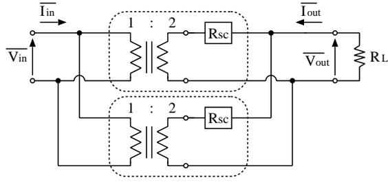
Fig.6 Equivalent circuit of proposed converter.
