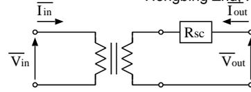
Fig.5 Equivalent circuit of step-up SC converter.
