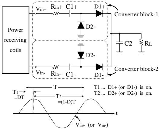
Fig.1 Conventional AC-DC converter.
