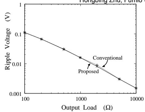
Fig.9 Simulated ripple voltage.
