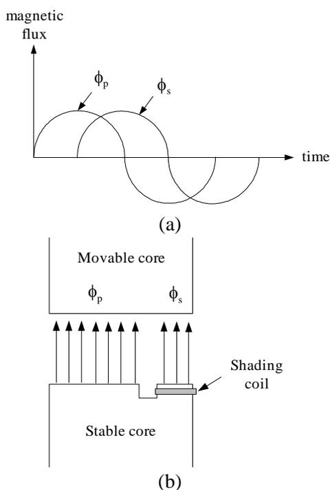
Fig. 2. Magnetic flux in the magnetic circuit (a) varies with time (b) mechanical distribution.
