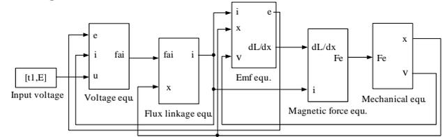
Fig. 5. Complete electromagnetic contactor model.
