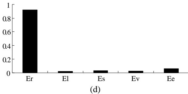
Fig. 8. Dissipated energy comparisons in each subsystem for the coil is energized by an ac source with initial voltage phase at (a) 0 degree (b) 45 degree (c) 95 degree (d) 135 degree.
