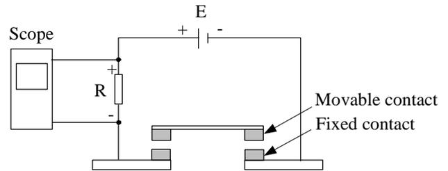
Fig. 9. Experimental rig for measuring the contact bounce during closing process.
