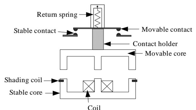
Fig. 1. Basic configuration of an ac contactor.
