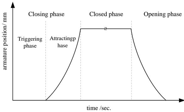
Fig. 3. Operating divisions of a contactor.
