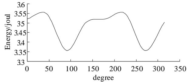
Fig. 7. Input power energy varies with initial voltage phase of applied coil voltage.
