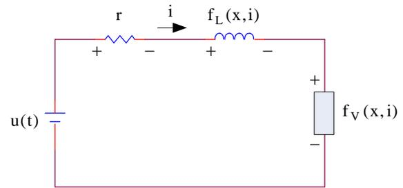
Fig. 4. Equivalent electrical circuit of a contactor.
