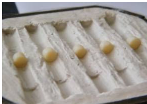
Fig. No 15. Composite cylinders aligned in the mould each of the mould patterns
