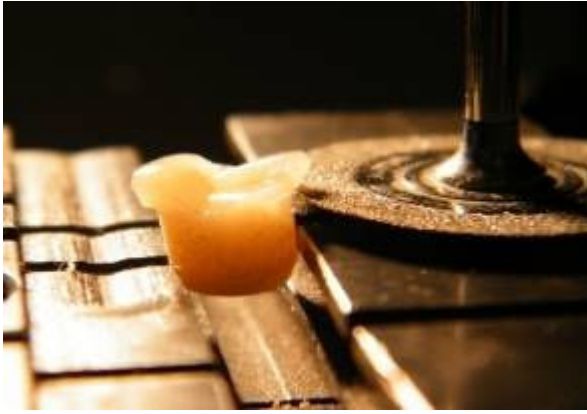
Fig. No.7. Aspect regarding the milling of the second base of the composite cylinder
