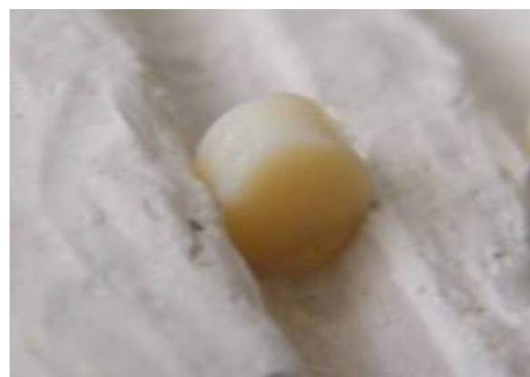
Fig. No 16. Composite cylinder placed in each mould patterns.
