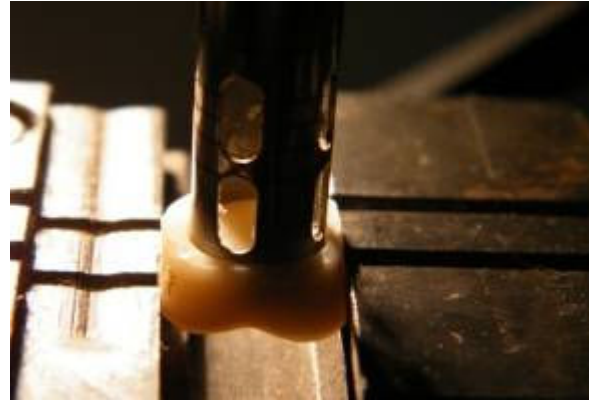
Fig. No 4. Mucosal view of the cylinder milled with the trepan bur inside the composite tooth.
