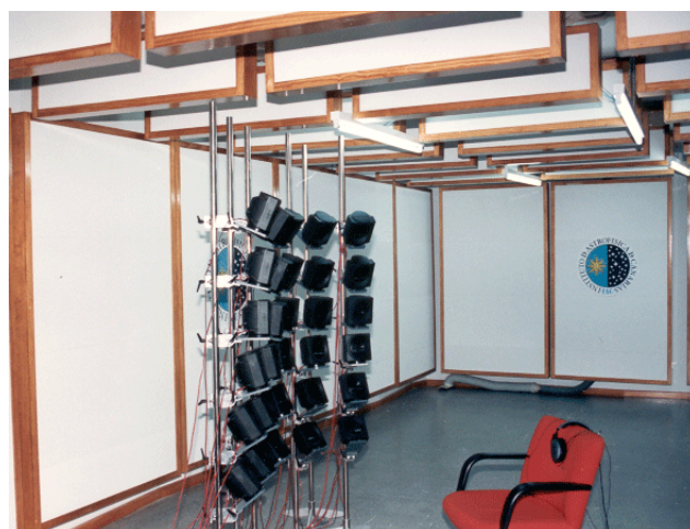
Fig.2. Loudspeakers array inside the acoustically prepared experimental room
