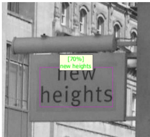
Fig.10. Example of a text both detected and recognized by the portable version of the reading system (green letters inside the white box)
