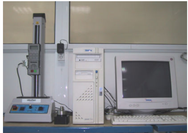
Fig. 4. Equipment for the traction test.
