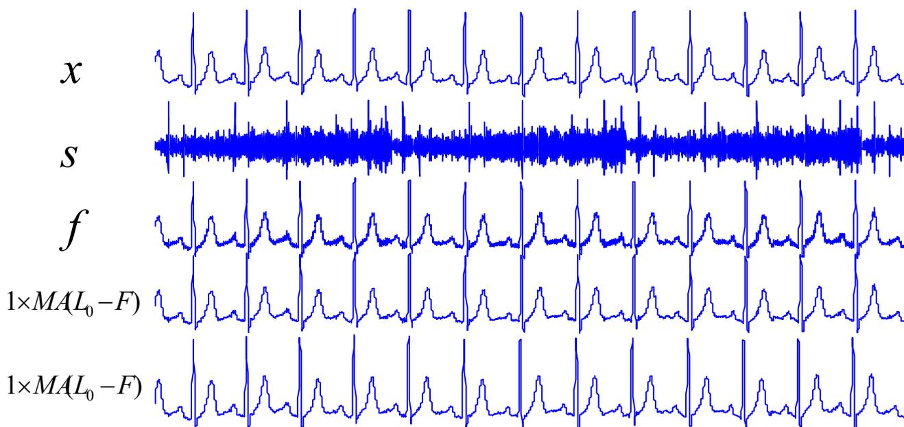
Figure4. Filtration of (ECG) signal by MA (Lo.F)  $1 \times MA(L_0 - F)$  one time and  $3 \times MA(L_0 - F)$  three times)
