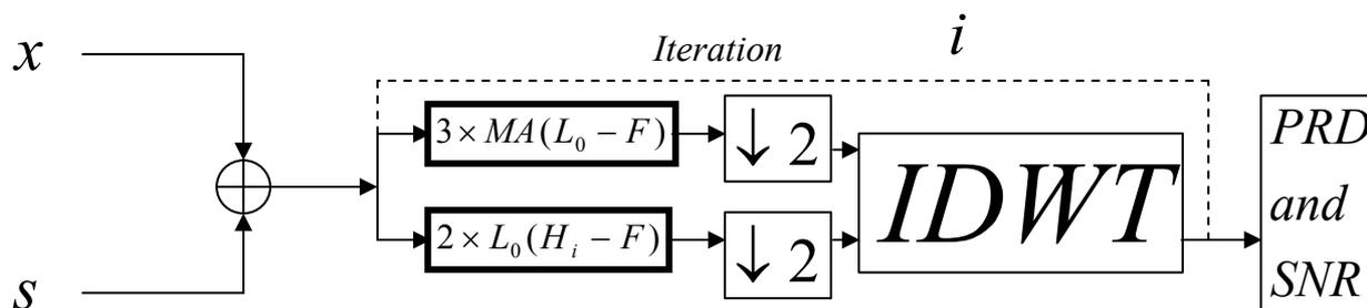
Fig. 5 The filtration system using MA (Lo-F) and MA (Hi-F) filters, where (i) is the number of the system repeating (iteration)
