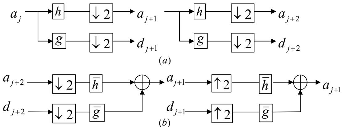
Fig. 3 Filter bank trees of a) Decomposition (DWT) and b) Reconstruction (IDWT)
