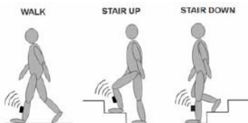
Fig. 1. Monitored activities, and sensor placement
