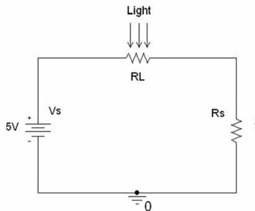
**Fig. 2.** The photoelectric conversion circuit of cone cell.
