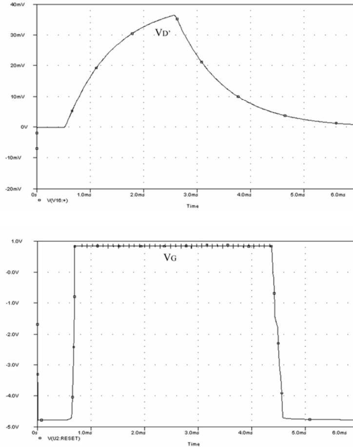
**Fig. 8.** The waveforms of  $V_D$  and  $V_G$ .  $V_D$ , the input of the voltage comparator U5A;  $V_G$ , the output of the voltage comparator U5A.
