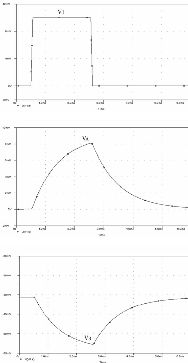
**Fig. 4.** The waveforms of  $V_1$ ,  $V_A$ , and  $V_B$ .  $V_1$ , the square wave plus as stimulation source;  $V_A$ , the capacitor C1 voltage;  $V_B$ , the cone cell potential.
