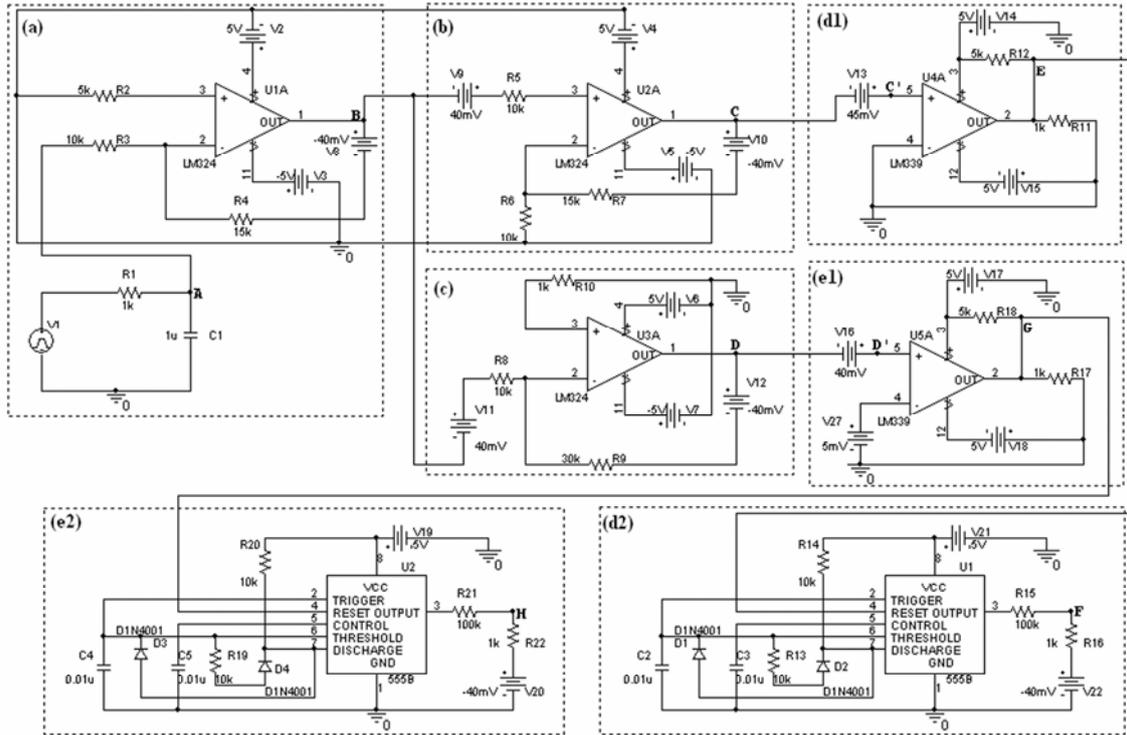
**Fig. 3.** The electronic circuit model of cone cell pathway in the primate while a light flash shines the center of receptive field. (a) Hyperpolarization circuit of cone cell. (b) Potential transmission circuit of off-center bipolar cell. (c) Potential transmission circuit of on-center bipolar cell. (d1) and (d2) Action potential generation circuit of off-center ganglion cell. (e1) and (e2) Action potential generation circuit of on-center ganglion cell.
