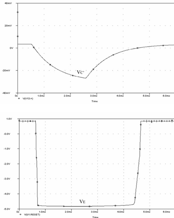
**Fig. 6.** The waveforms of  $V_{C'}$  and  $V_E$ .  $V_{C'}$ , the input of the voltage comparator U4A;  $V_E$ , the output of the voltage comparator U4A.
