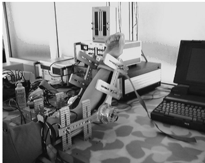
Fig. 2: The isometric brace used to keep the elbow angle constant at 120^\circ during the isometric acquisition of sEMG signals. Torque sensors are located at the joint of the rigidly connected parts of isometric brace.
