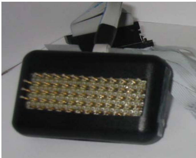
Fig. 1: Two-dimensional matrix (13 rows and 5 columns) of surface electrodes used for sEMG acquisition.
