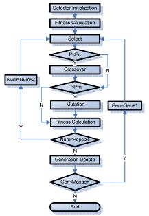
Fig. 1. Detector generation algorithm based on GA
