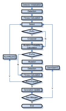
Fig. 2. Detector generation algorithm based on online GA
