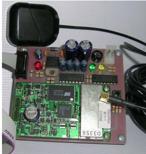
Fig. 4. GPS receiver engine board for report the position of patient.
