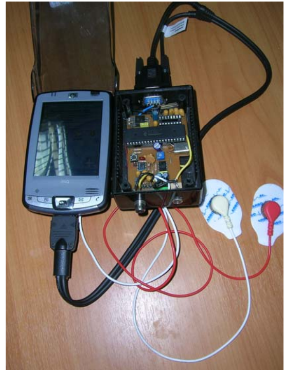
Fig. 6. The prototype of the PEM monitor.
